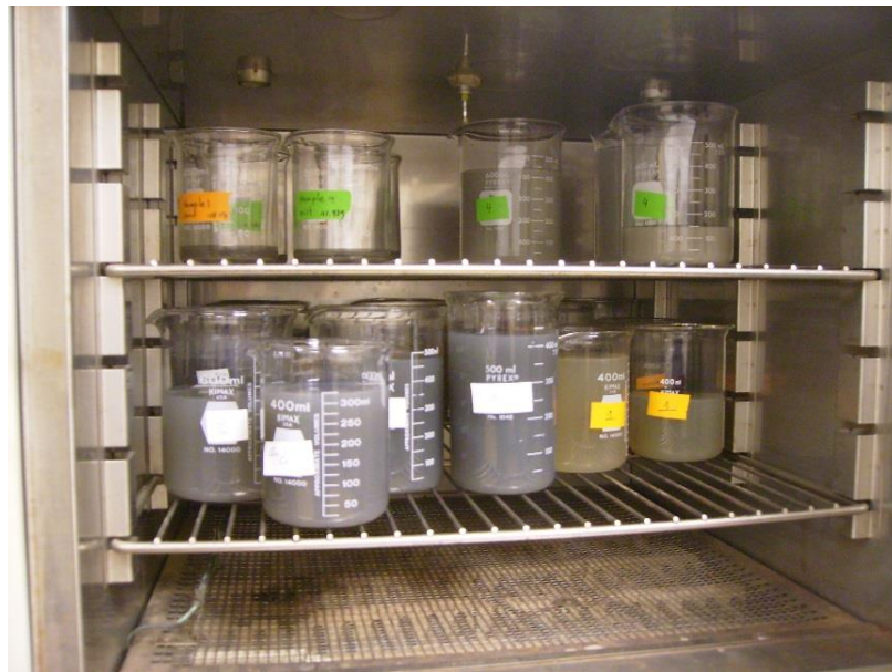
Figure A11. Supernatant that contained the clay in suspension in the oven at 40°C.
