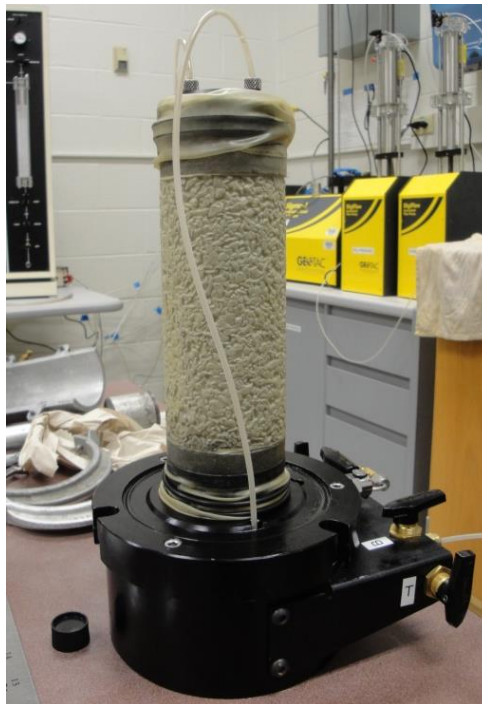
Figure 5.5. Dry compacted shale specimen. This sample is under vacuum pressure. Notice the penetration of the membrane in the specimen.
