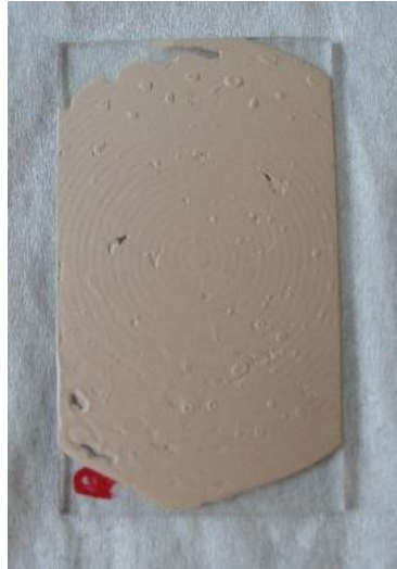
Figure 3.4. Slide with sample after pretreatment used to run the XRD test.
