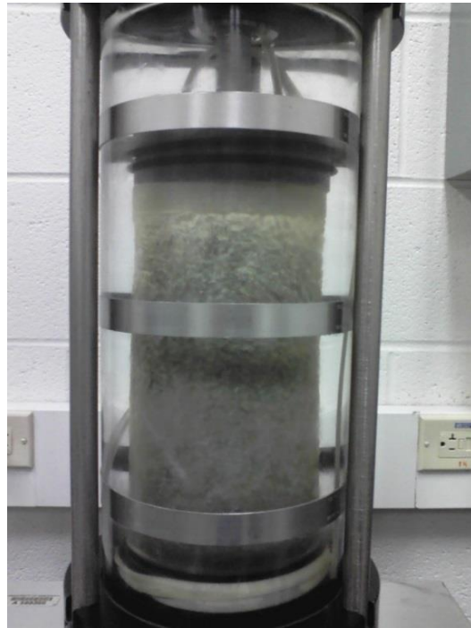
Figure 5.7. Specimen during the soaking.
