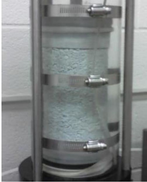
Figure 5.11. Appearance of the specimen after the Isotropic Consolidation.
