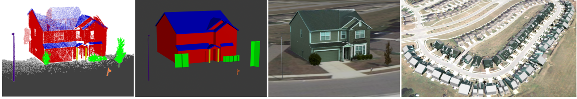
Figure 5.1: The pipeline of semantic segmentation and reconstruction of LiDAR point clouds. From left to right: (a) semantically labeled 3D point cloud; (b) reconstructed objects using category-specific methods, including billboard trees, replaced common objects, and a building. The color-code on the building shows recognized different building parts; (c) textured 3D models on a ground plane, and (d) an overview of an automatically reconstructed large-scale scene.
