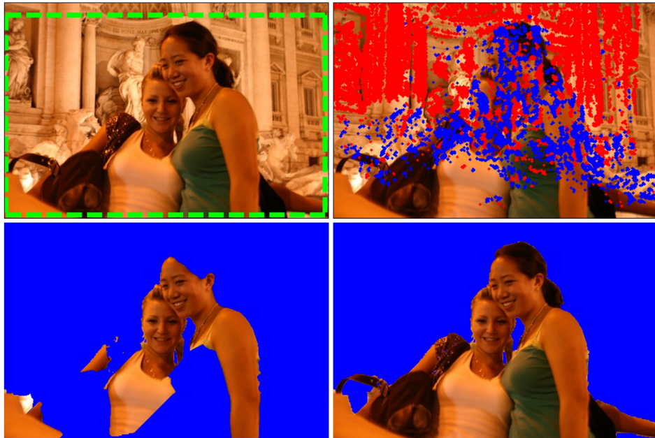
Figure 4.2: Segmentation results: (top left) the original image superimposed with the bounding box prior for Grabcut, (top right) red dots for background color seeds and blue dots for foreground color seeds, (bottom left) the result of Grabcut, (bottom right) the result of our automatic approach.
