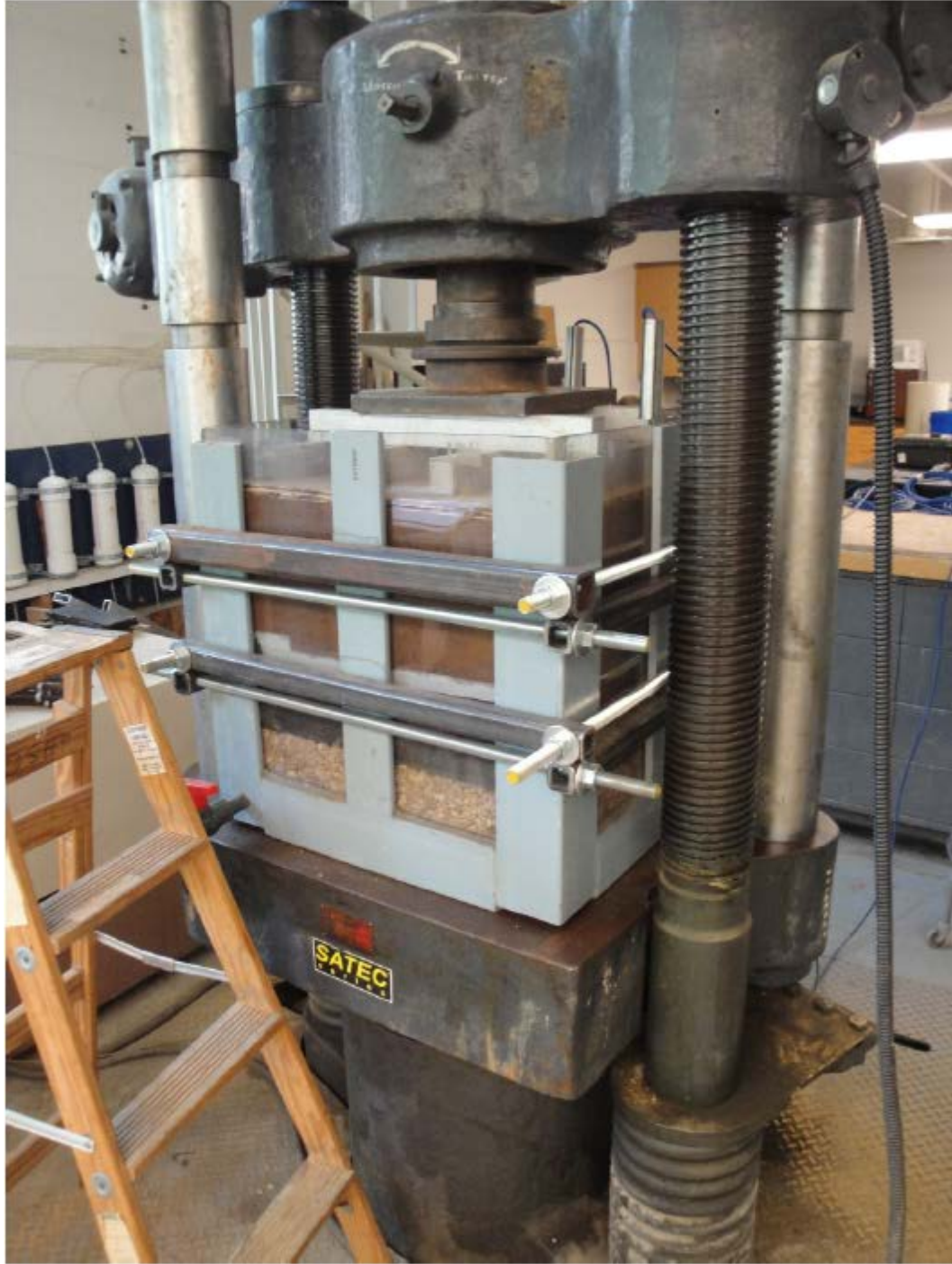
Figure C.3 Large box test setup (Huff, 2010).
