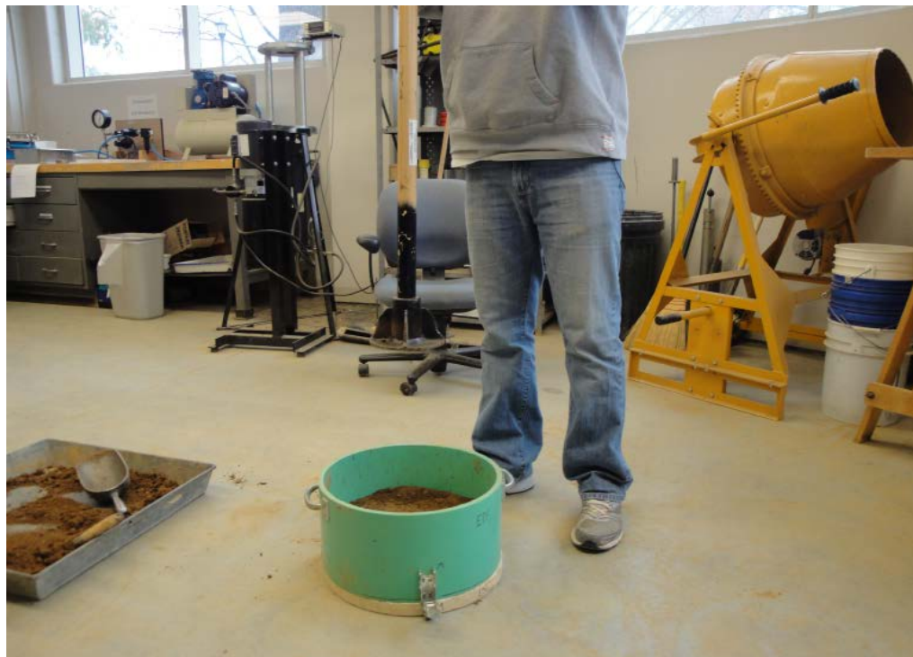
Figure 2.4: Manufacturer suggested mold and hammer
