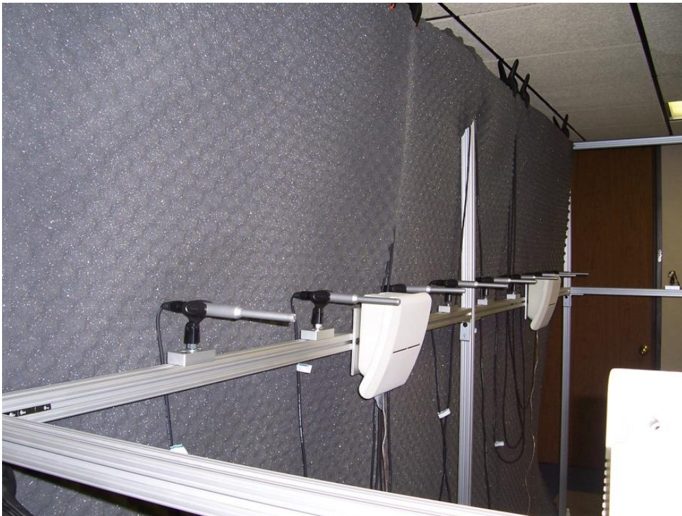
Figure 6.1: Cage side with Linear Microphone array, a couple of speakers, and absorptive acoustic treatment
