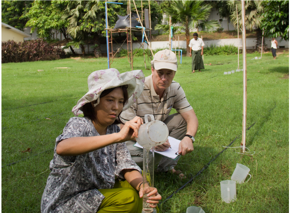
Rowell and his Burmese counterpart, Mar Lar Soe, measure drip irrigation system uniformity in a test plot on the grounds of Rangoon's 2500-year-old Shwe Dagon Pagoda.
