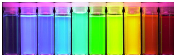
Figure 1-2. Quantum dot fluorescence spanning the visible spectrum. Although not shown here, some formulations emit in the NIR bioimaging window. Adapted with permission from Elsevier, Copyright © 2009 16 .
