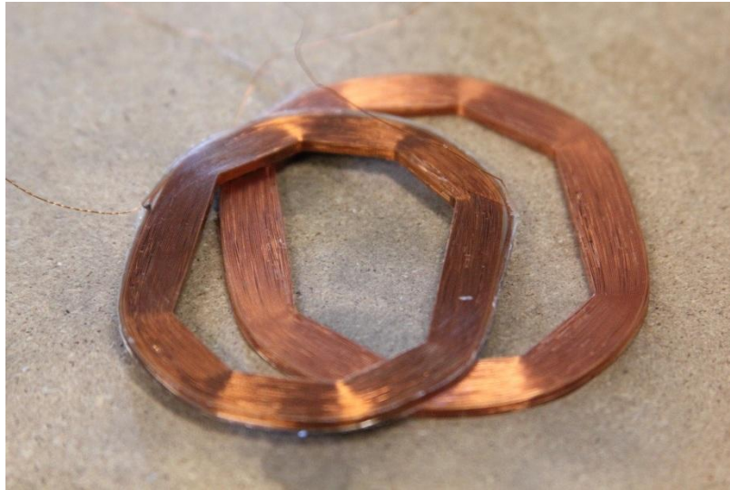
Figure 8: An example of magnetorquers. Note that they are essentially tightly wound coils of wire that become an electromagnet when energized. Source: Wikimedia Commons
