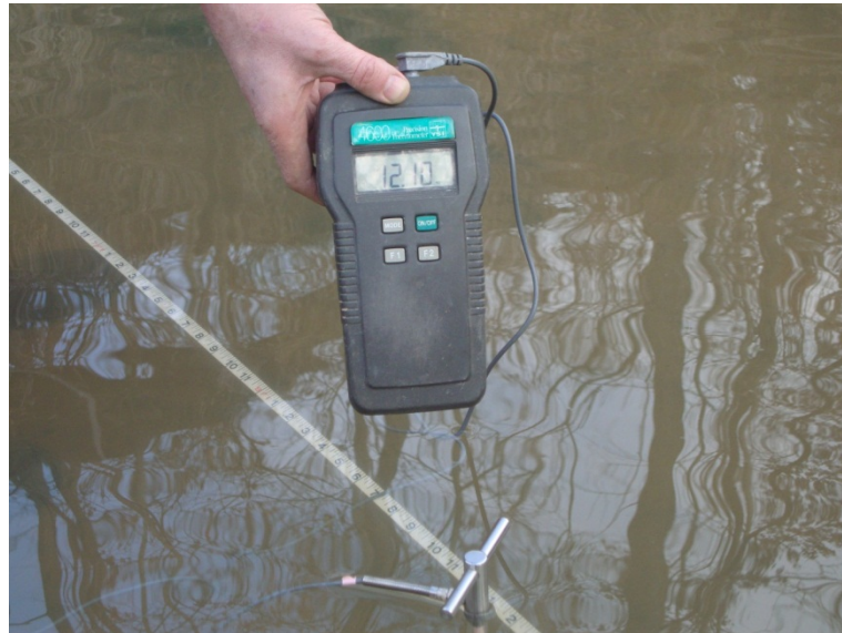
Figure 2.4. Temperature probing in January 2011 showing groundwater inflow location with anomalously higher temperature ( 12.10^{\circ}\text{C} ) when the average stream temperature was 4^{\circ}\text{C} .
