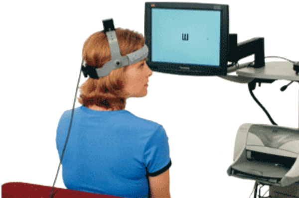
Figure 4.3 Example of the head mounted tracker and optotype stimulus. Used with permission
