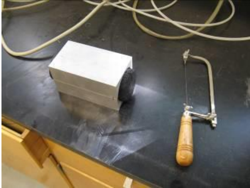
Figure B.10: Trimming the ends of the sample.
