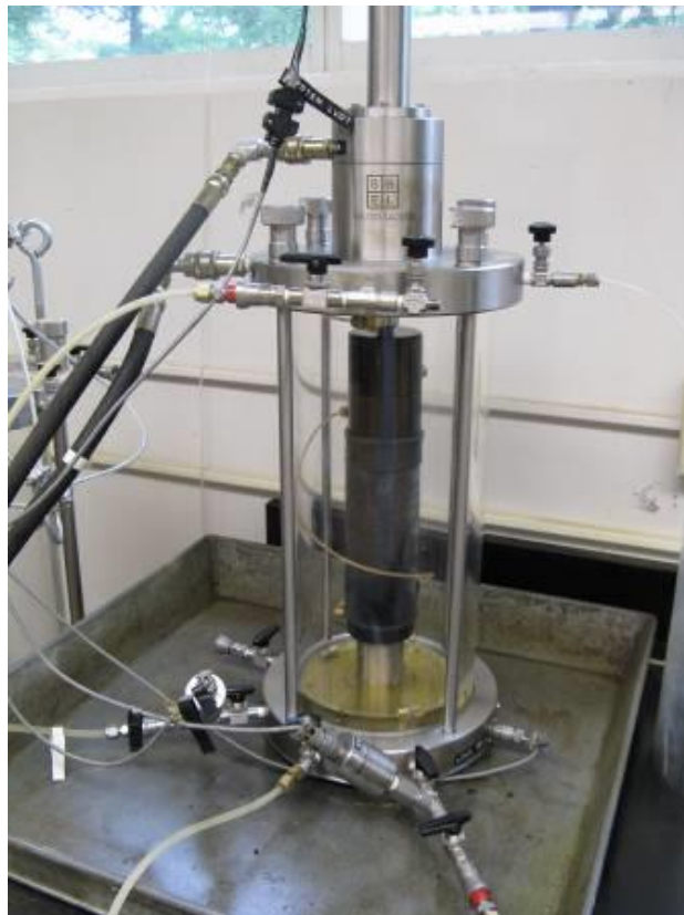
Figure B.14: Filling the chamber with oil.
