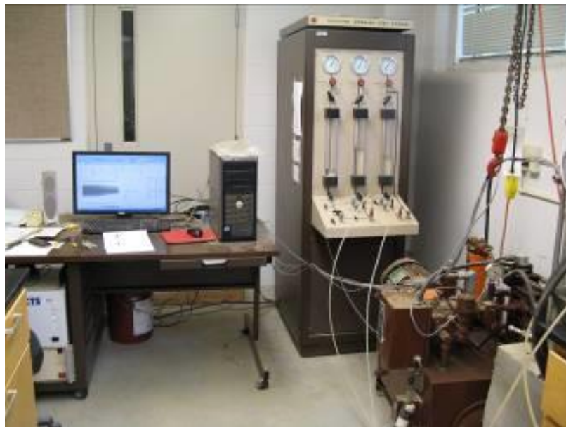
Figure B.1: pressure board, hydraulic pressure generator, personal computer, and the controlling computer.
