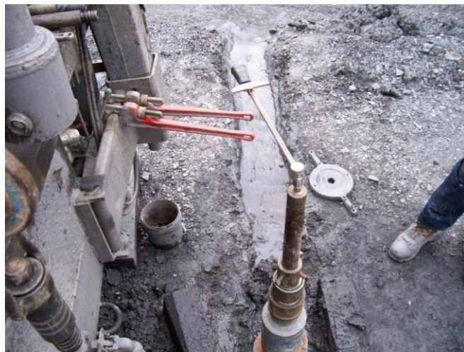
Figure 2.18: Measuring in-situ undrained shear strength using a torque wrench.
