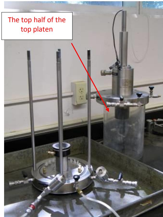
Figure B.11: The top half of the top platen is secured to the loading rod.
