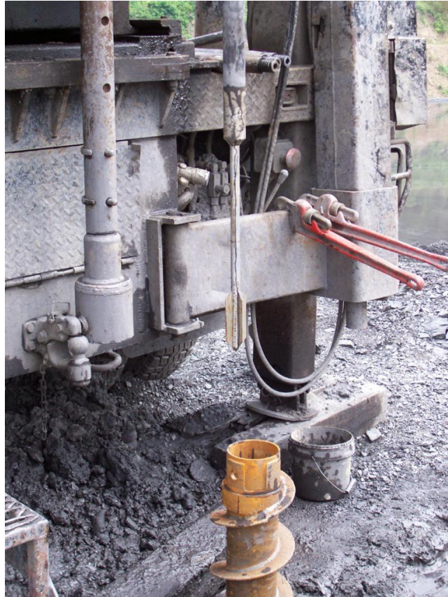
Figure 2.17: Tapered vane used for in-situ vane shear test.
