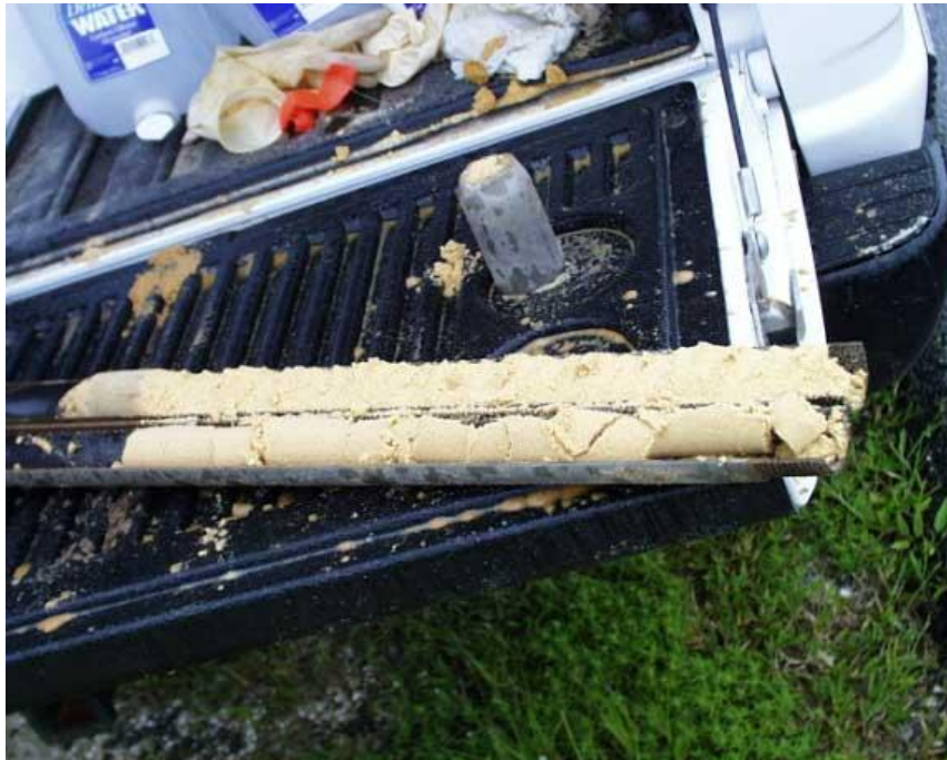
Figure 2.14: An example of the SPT sampler and the obtained disturbed sample.
