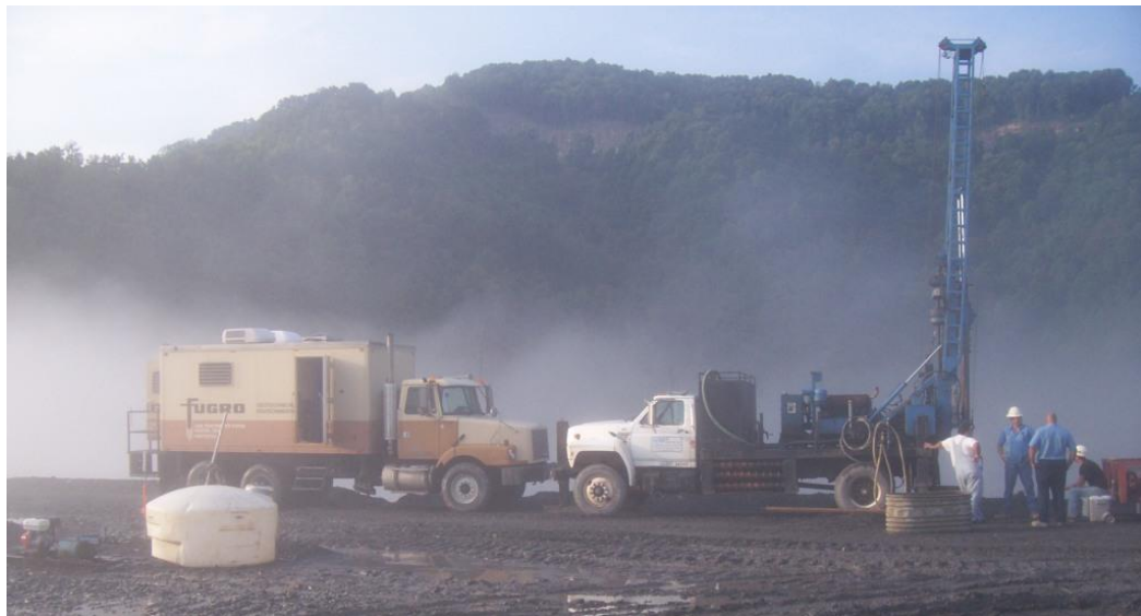
Figure 2.2: Performing sCPTu and SPT testing at location A (crest) at Abner Fork.
