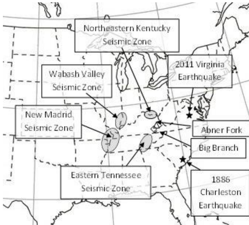
Figure 1.11: Location of the selected tailings impoundments in this study, the nearby seismic sources and historic seismic events.
