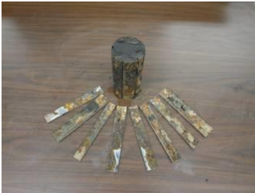
Figure B.6: Cutting the tube with an electric saw.
