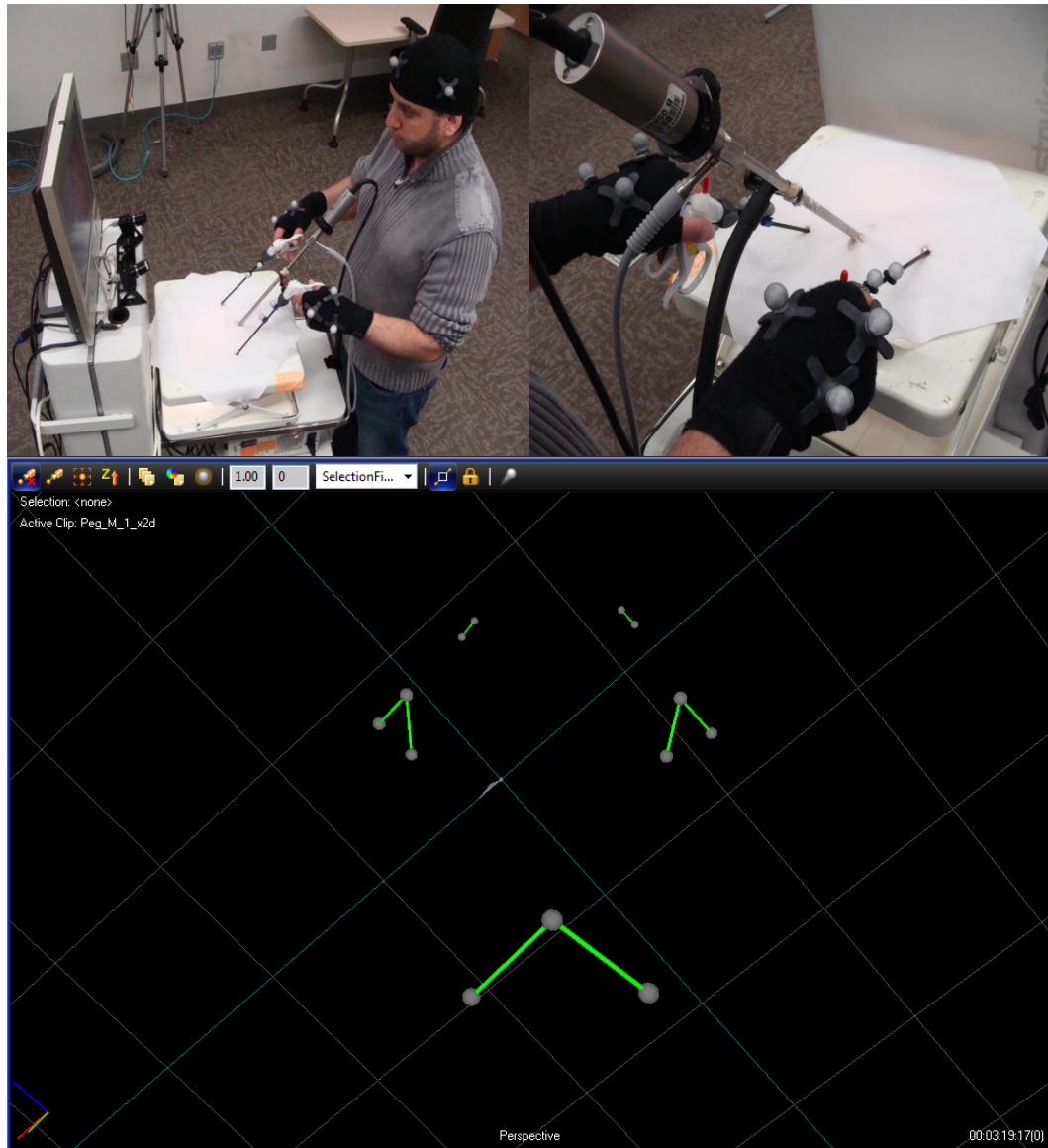
Figure 3.14 Template of markers used to track 3D positions and rotations of the subject's head, hands, and the surgery tools. The top two pictures show the real markers and the bottom one shows the markers' resolution from top view.
