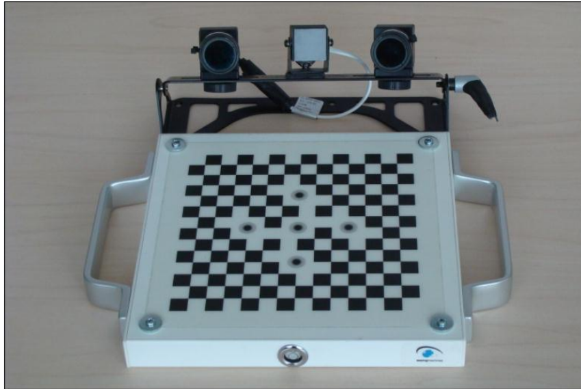
Figure 3.15 FaceLAB eye tracker cameras with calibration kit
