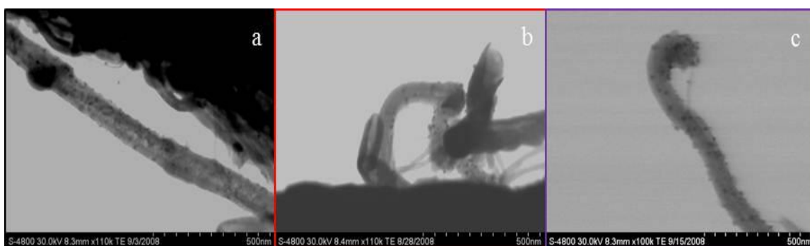
Figure 2-7 STEM images of (a) as-prod-N-MWCNTs and products of complexation reaction; (b) 2-38 and (c) 2-39 of scheme 2-2.
