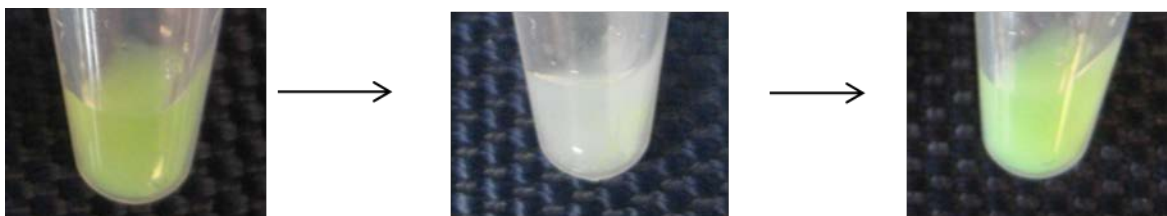
Figure 7.12 Reversible immobilization of sfGFP-SSB on NHS-resin. NHS-dT 37 resins modified with sfGFP-SSB (left), eluted using dA 35 (middle), and then regenerated and incubated with fresh sfGFP-SSB (right).
