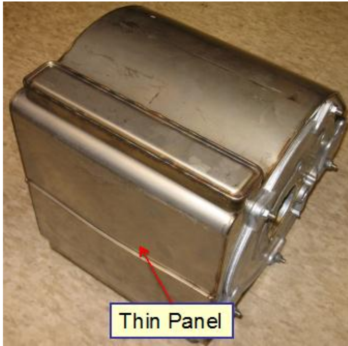
Figure 3.42 Combustion chamber with thin and nearly flat panel.
