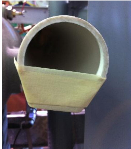
Figure 2.11 Photograph showing partially blocked intake.
