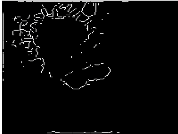
Fig. 5-5 Droplet edges detected by the Sobel operator
