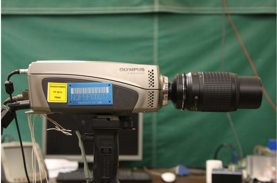
Fig. 4-5 Second high speed camera for image recording and off-line analysis
