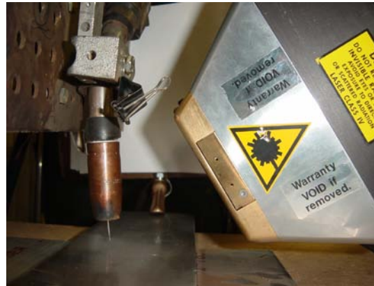
Fig. 2-15 Installation of GMAW and Laser (the shielding board is not shown in the picture)
