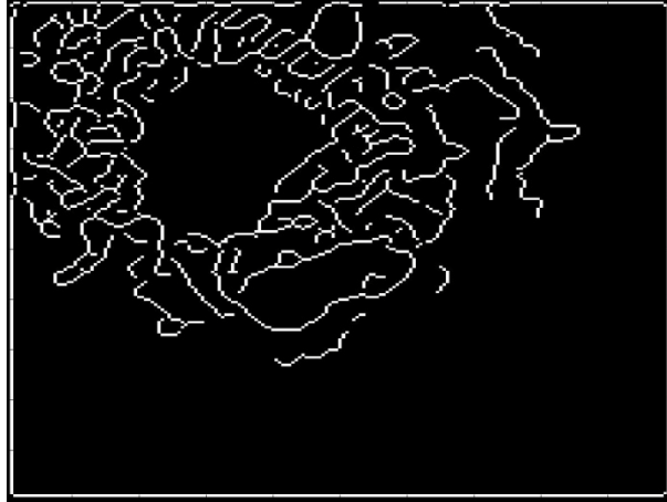
Fig. 5-6 Droplet edges detected by the Canny operator
