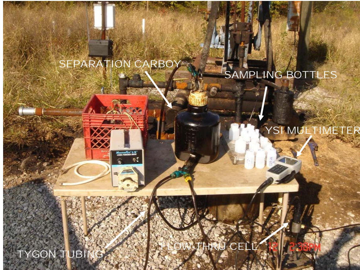
Figure 3.1 Photo showing the field setup apparatus used to sample formation waters. Oil was separated from formation water in the separation carboy. The outflow water from the separation carboy was further filtered before entering the flow-through cell for the YSI multi-meter. The large waste carboy on the ground collects overflow (photo by G. Beck, 2009).
