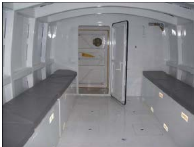
Figure 1.9. Inside of Steel Refuge Chamber
