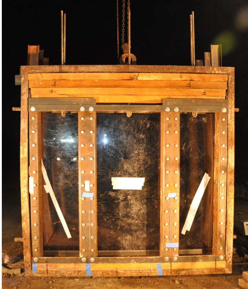
Figure 3.21. Constructed Smaller Polycarbonate Wall System for Additional Testing
