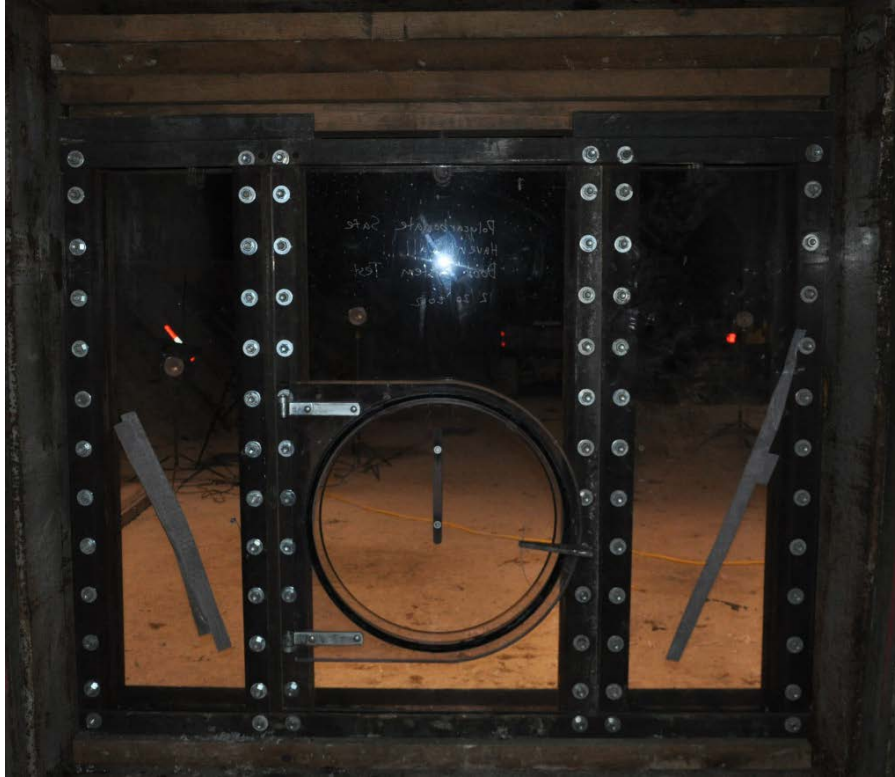
Figure 3.31. Installed Door System for Testing (Outside)
