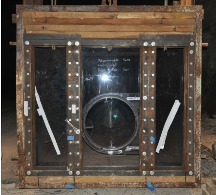
Figure 3.29. Installed Door System for Testing (Inside)
