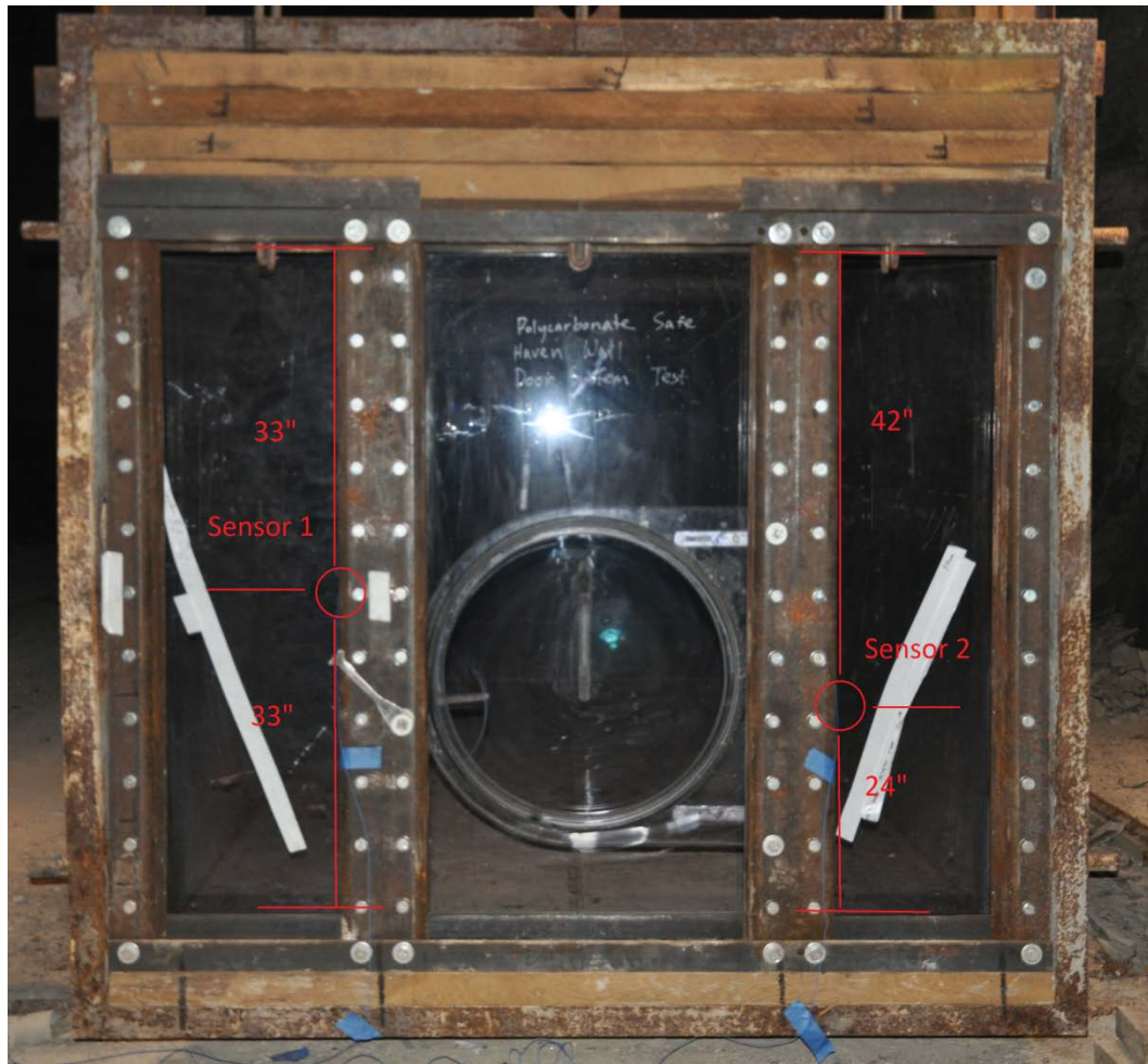
Figure 3.33. Sensor Arrangement for Door Testing
