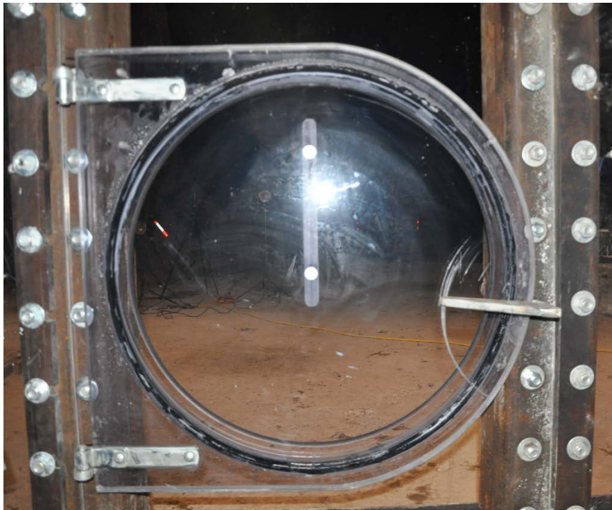
Figure 3.32. Installed Door (Outside)
