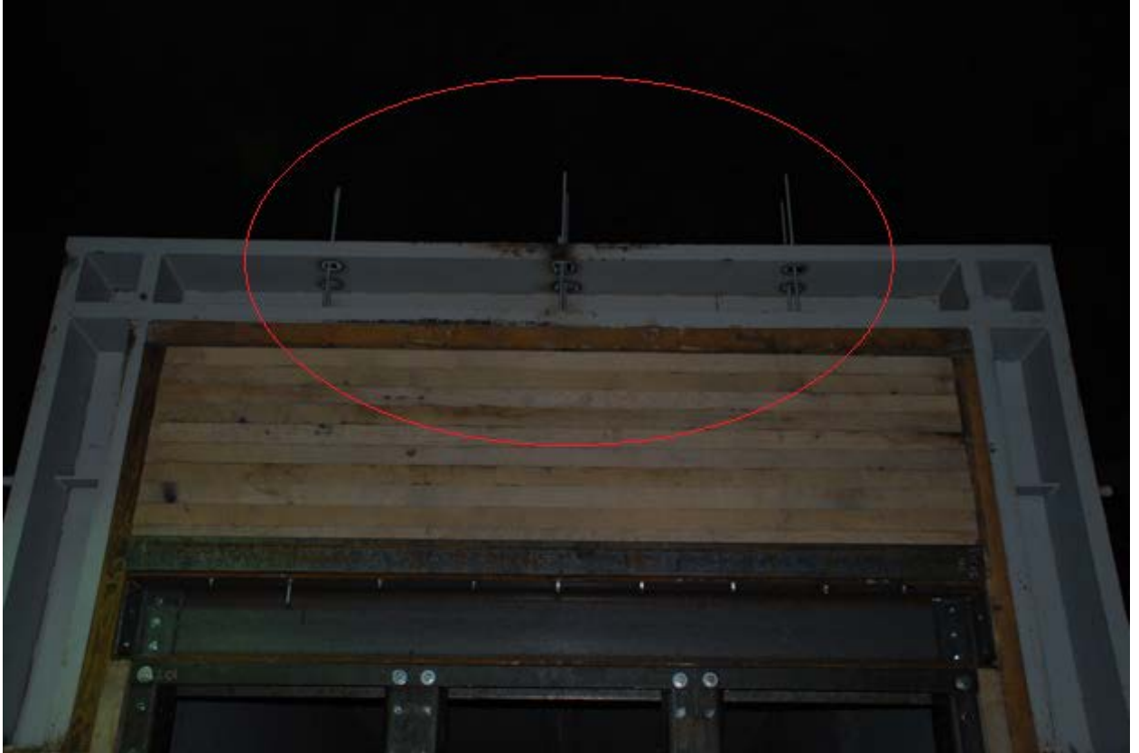
Figure 3.3. 5/8 inch Threaded Steel Bars Through Boards and I-beam
