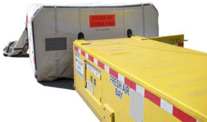
Figure 1.6. Fresh Air Bay Inflated Out of the Fresh Air Bay Skid
