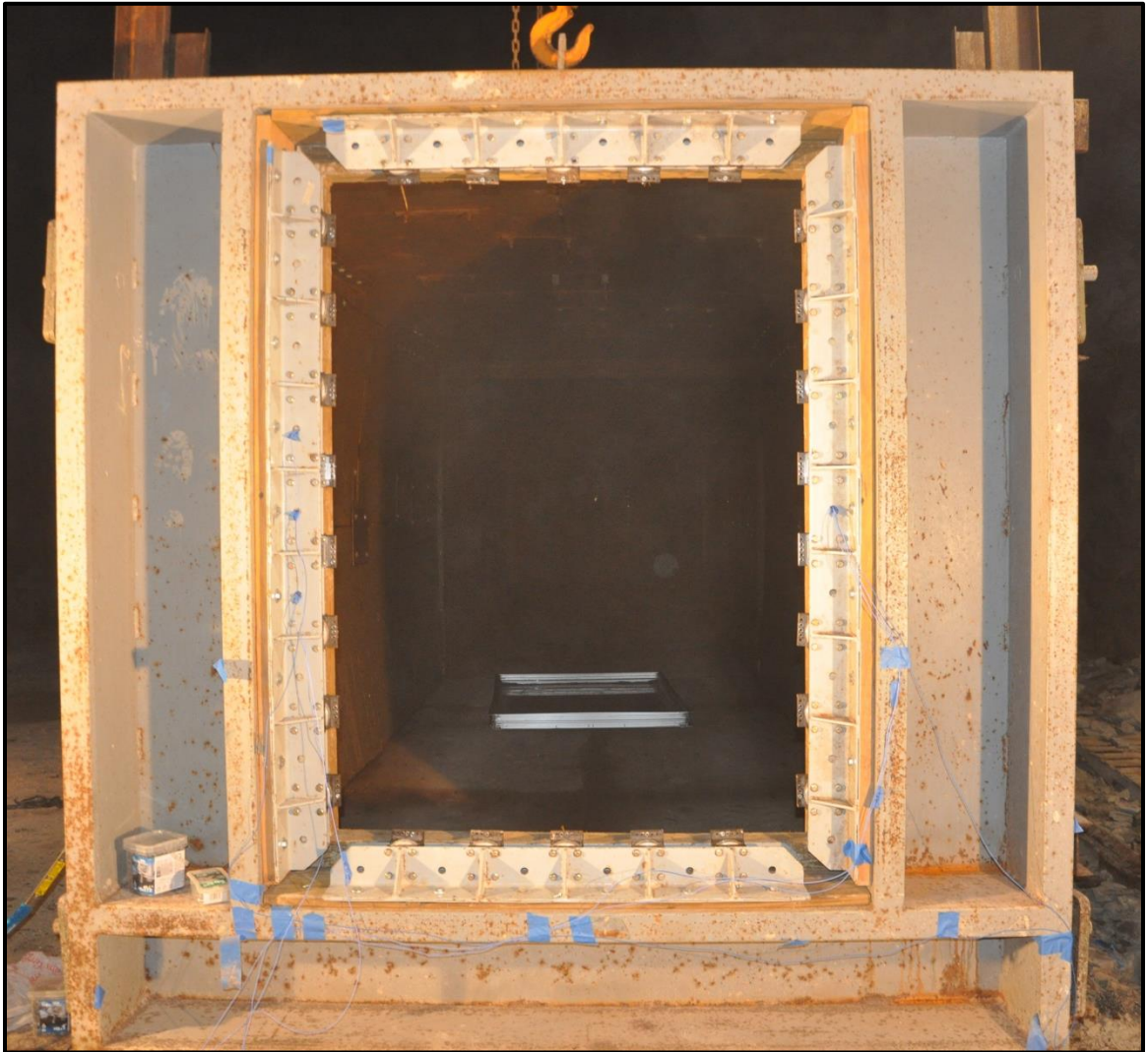
Figure 7.2: 1/2 inch polycarbonate sample post-failure
