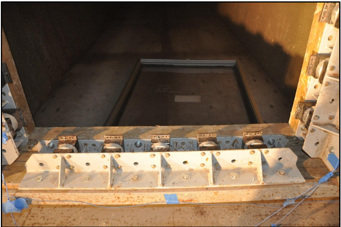
Figure 7.1: 1/4 inch polycarbonate post-failure
