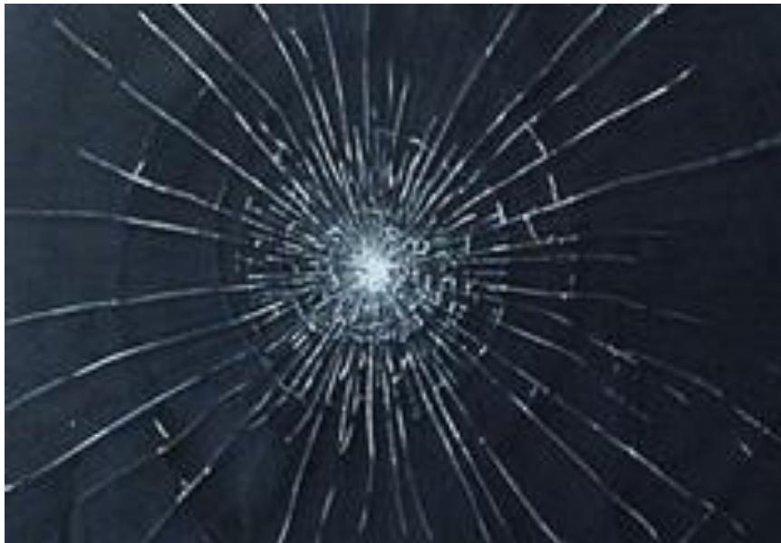
Figure 2.5: Laminated glass breakage pattern (Stiles, 2010)
