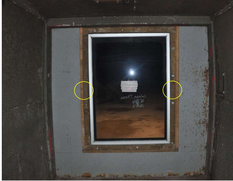
Figure 3.1: Mounting location of piezoelectric dynamic pressure
