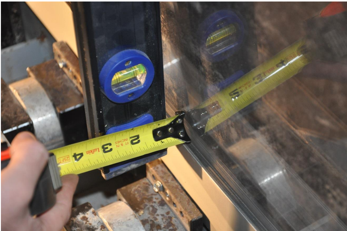
Figure 5.4: Residual deflection of 1/4 inch polycarbonate after perimeter testing.
