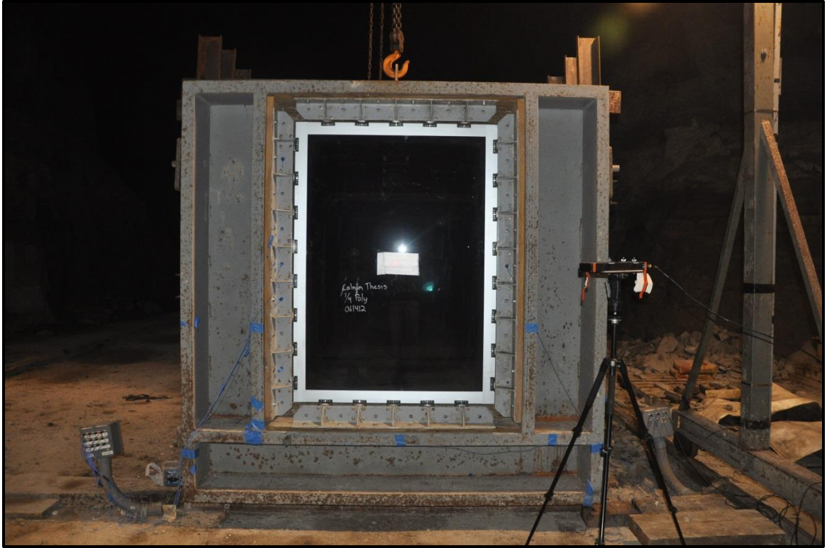
Figure 3.6: Buck fully prepared for testing
