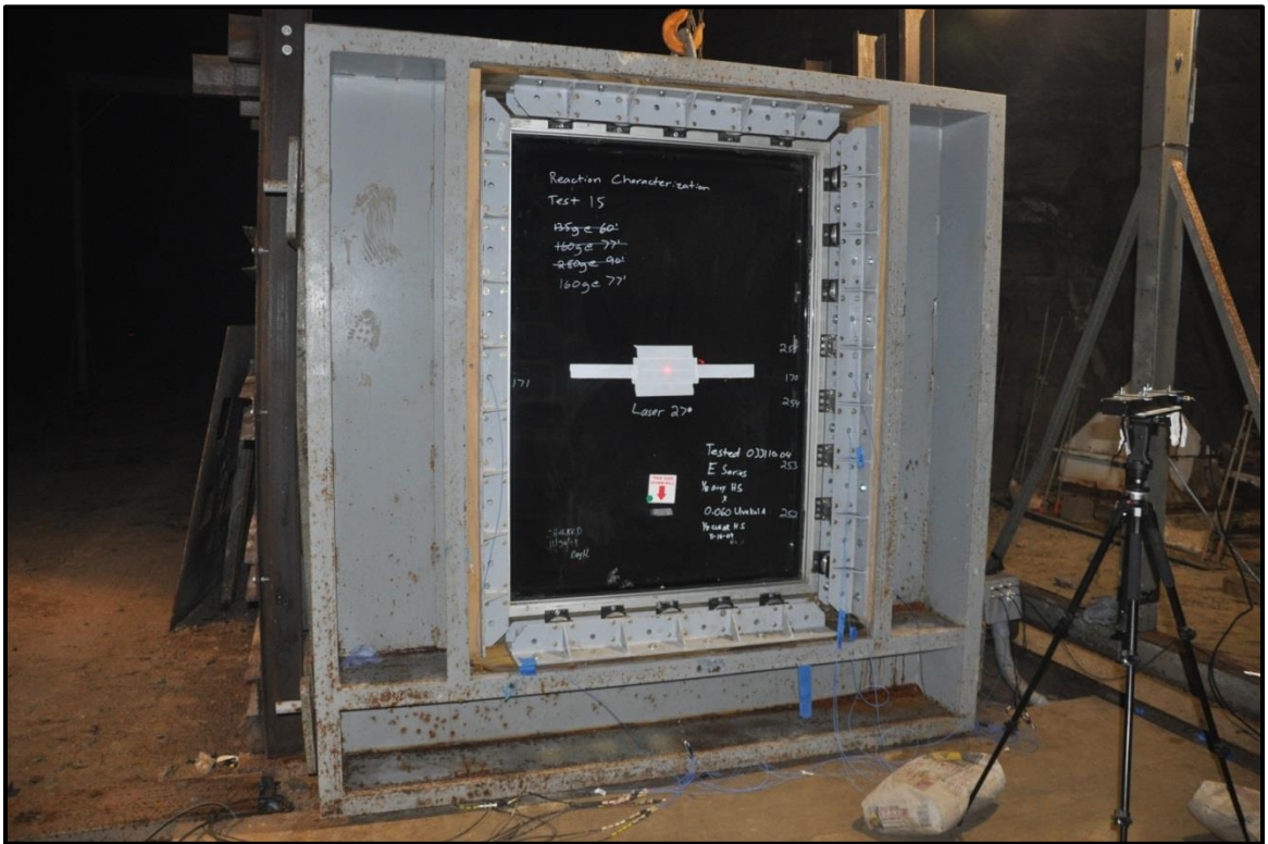
Figure 9.1: Laminated glass blast-resistant glazing system installed in buck (W.C. Wedding, 2010)
