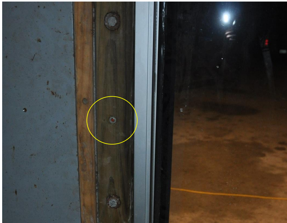
Figure 3.2: Detailed view of pressure sensor mounted in wood
