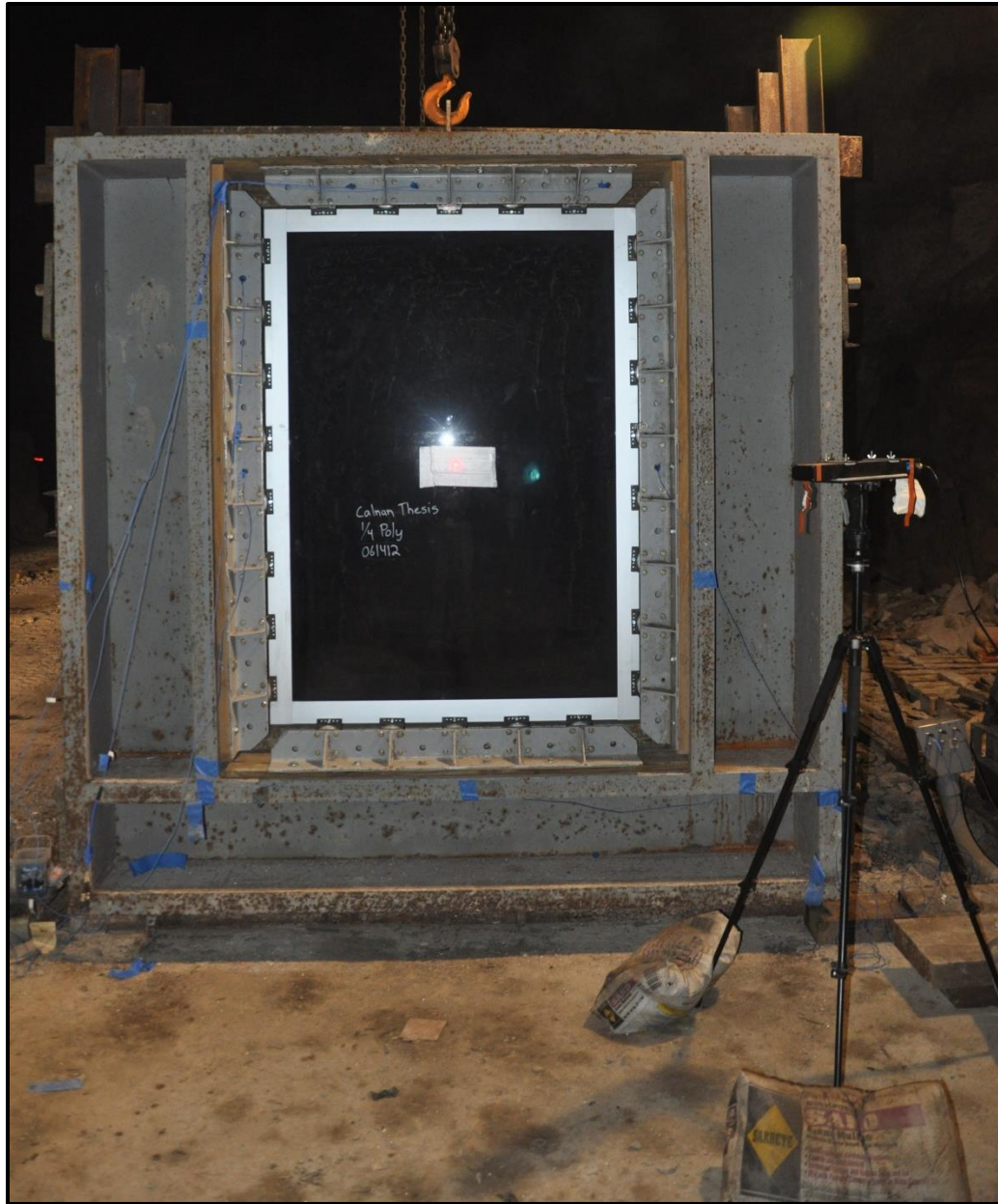
Figure 3.3: Laser distance gauge setup adjacent to the test sample
