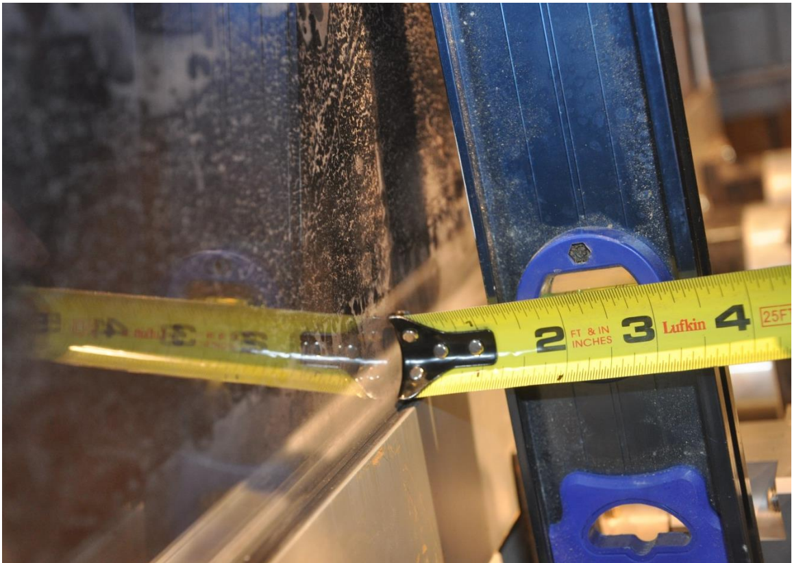
Figure 6.3: Residual deformation of 1/4 inch polycarbonate following repeatability testing.
