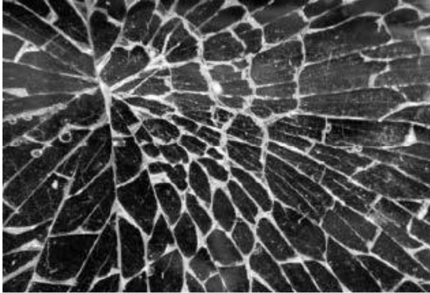
Figure 2.3: Tempered glass breakage pattern (Stiles, 2010)
