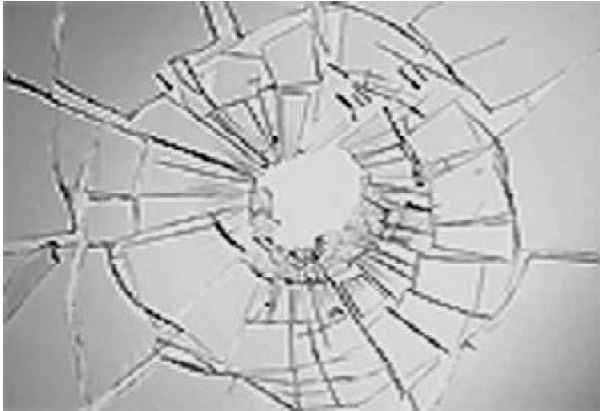
Figure 2.2: Annealed glass breakage pattern (Stiles, 2010)
