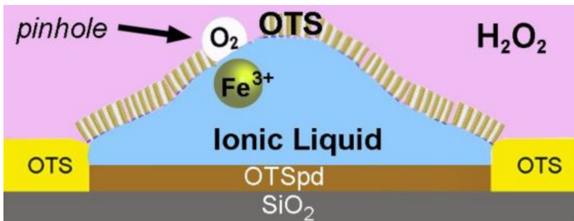
Figure 5-2 Octadecyltrichlorosilane (OTS)-coated ionic liquid/FeCl 3 drop.
