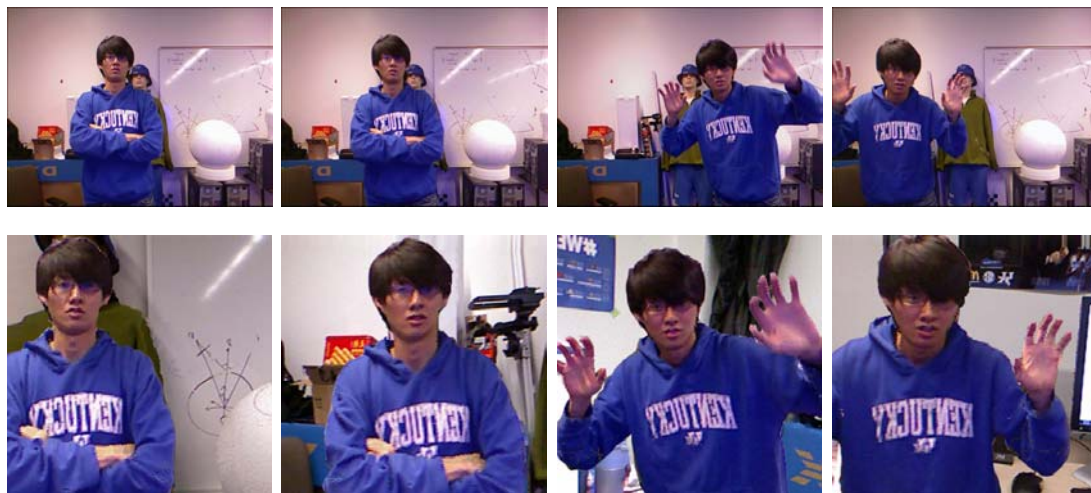
Figure 1.2: Mirror View Results: the first row contains the original RGB frames; the second row is the generated mirror view with virtual background; Images from the same column correspond to the same frame in the captured video sequence.
