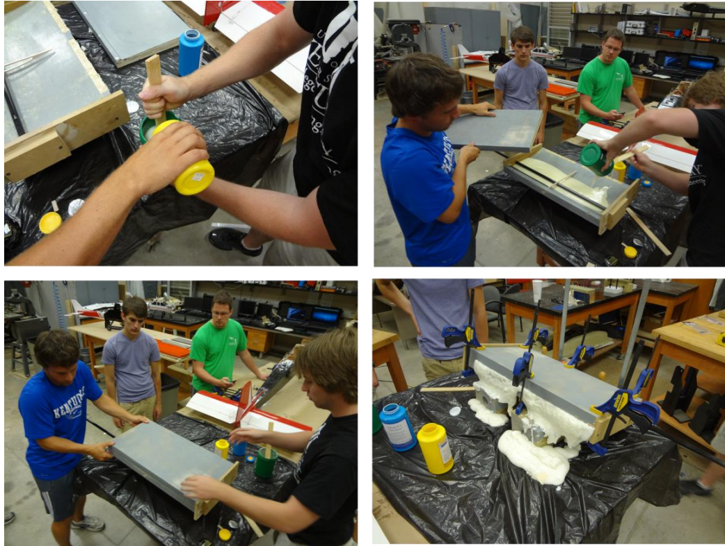
Figure 4-11: Manufacturing AB foam wing
