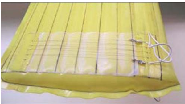
Figure 2-11: Left) Nitinol actuator for an inflatable wing-Right) Actuated and zero deflections [18]
