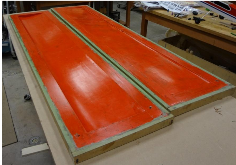
Figure 4-17: Female molds constructed of orange gelcoat and fiberglass
