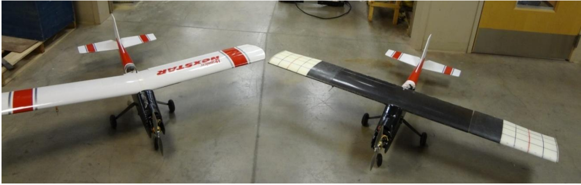
Figure 4-13: Wing warping wing and standard configuration wing on NexStar test bed
