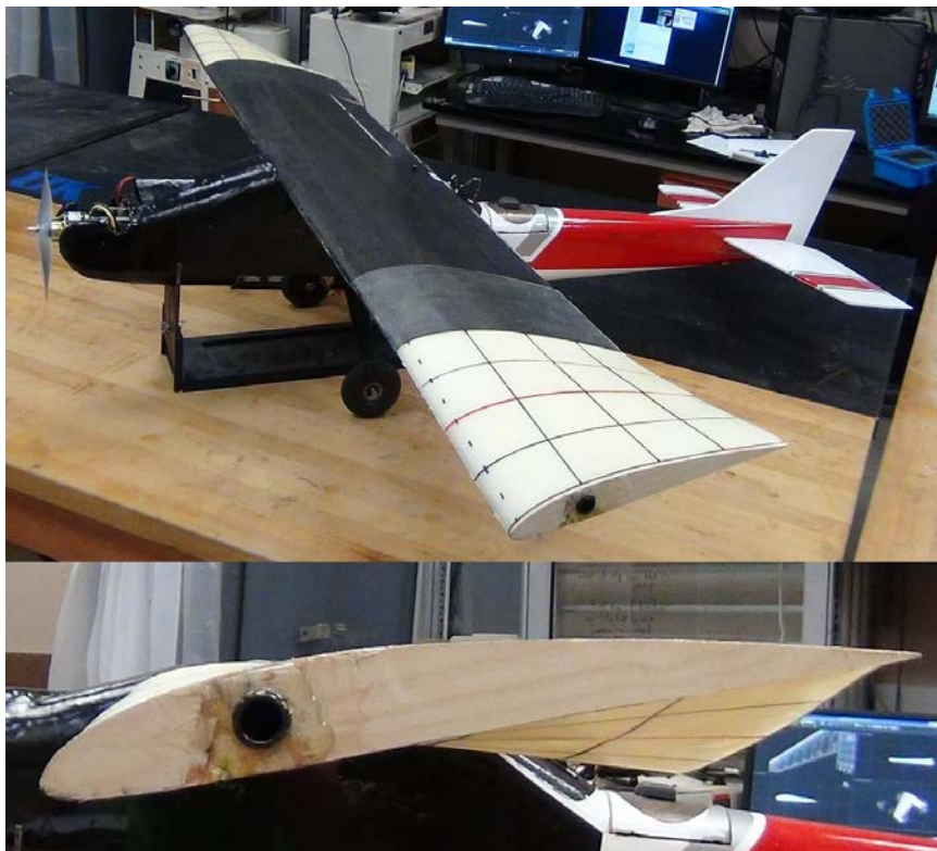
Figure 5.2 Twisting wing used in this study, \delta_a = -15^\circ
