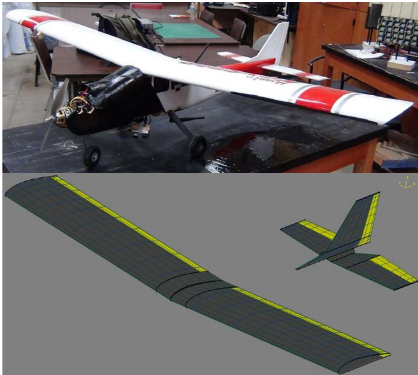
Figure 5.1 AVL model of a standard Hobbico® NexSTAR™ compared to the autonomous NexSTAR™
