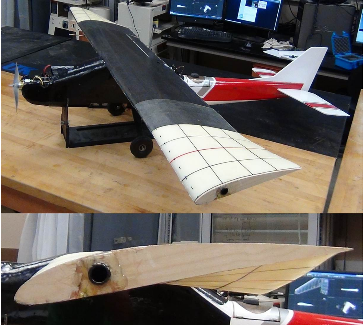
Figure 2.27 Recently developed wing shaping demonstrator used in this study
