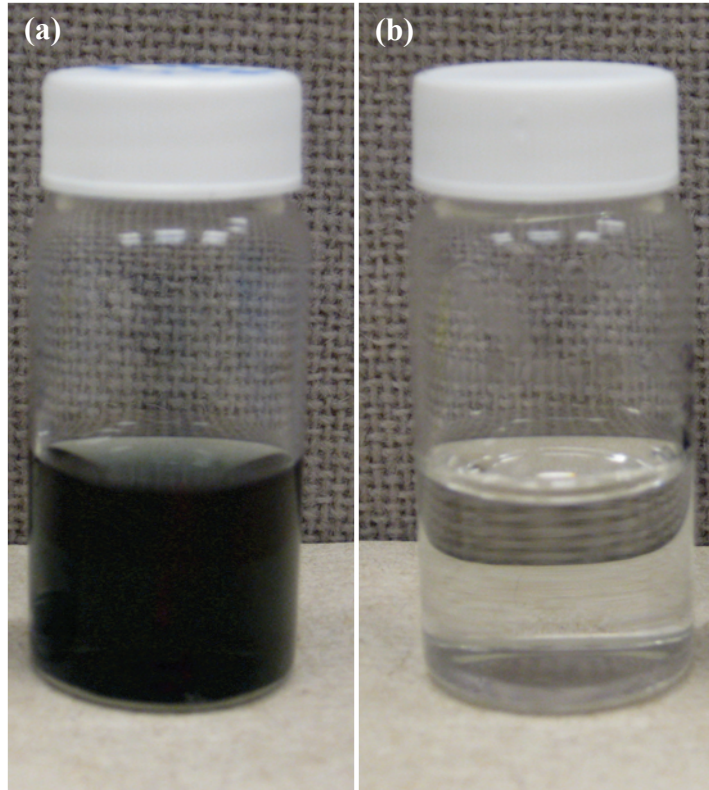
Figure 2.6 Suspended nano test tubes a) gold/titanium hybrid test tubes (50 nm x 1 \mu\text{m} dimensions) at a concentration of \sim 7 \text{ cm}^2 pillared replicas per milliliter b) pure titanium test tubes of the same size and concentration.
