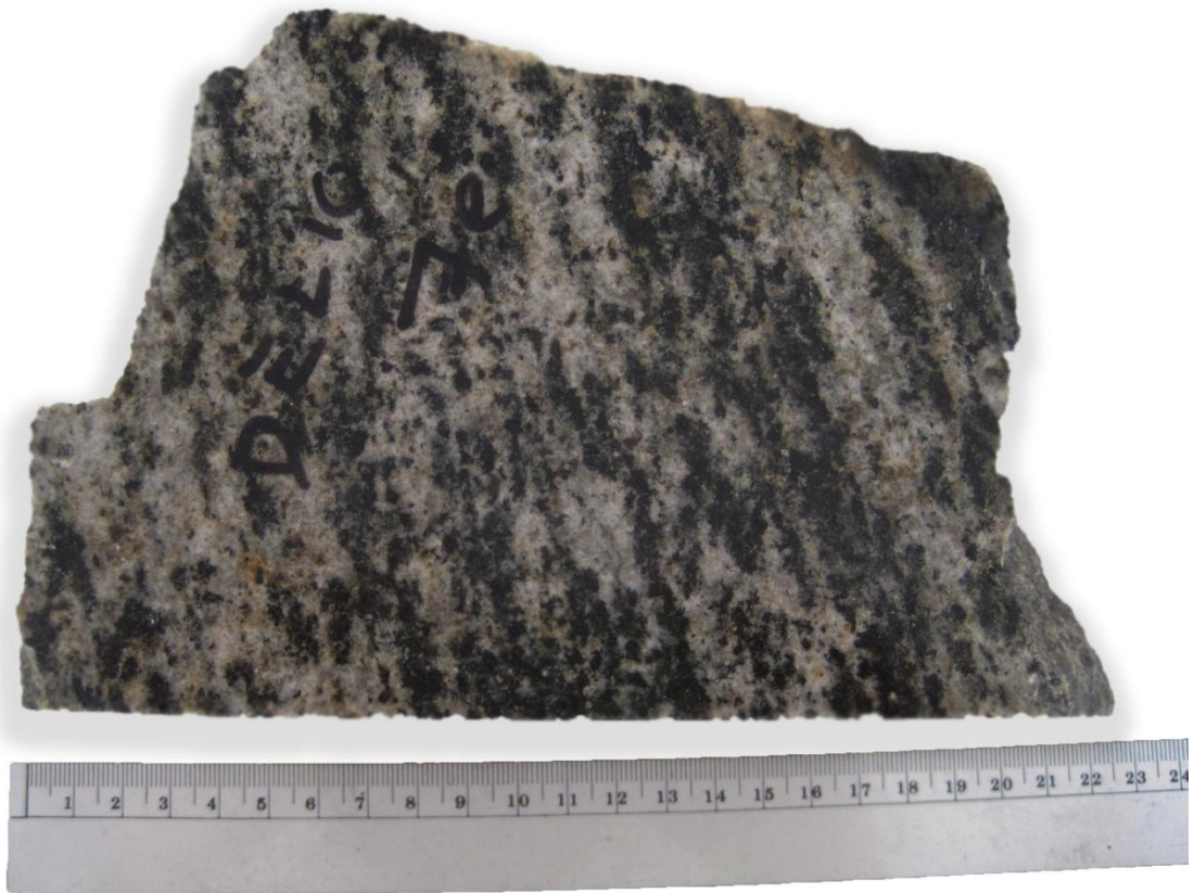
Figure 3.9: Slab cut parallel to lineation from hornblende gneiss sample DEL10-7e. Ruler units are in cm.
