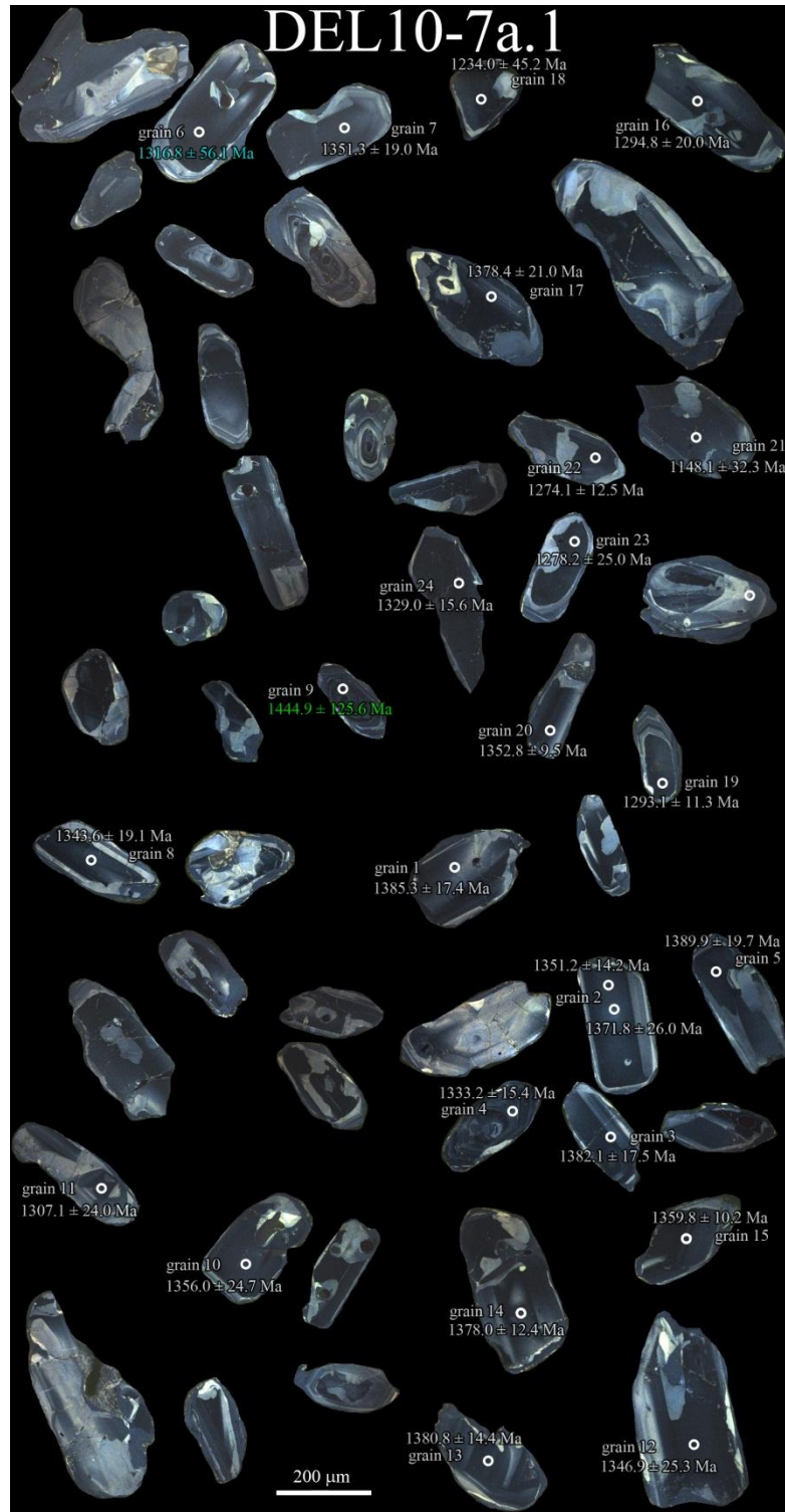
Figure 5.9: Cathodoluminescence images of zircon grains from sample tx-DEL10-7a.1. Rings represent 20 \mu\text{m} LA spot locations. Blue ages are analyses with more than 5 % reverse discordance. Green ages are analyses with anomalously high ^{204}\text{Pb} counts. These analyses were not included in the Concordia mean ‘best age’ plots. Errors are 1\sigma .
