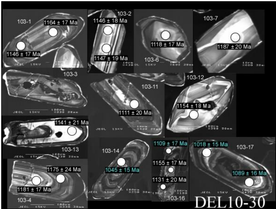
Figure 5.3: Cathodoluminescence images of zircon grains from agn-DEL10-30. Rings represent 30 \mu\text{m} SHRIMP II spot locations. Blue ages are analyses that were not included in the mean age calculation. Errors are 1\sigma .
