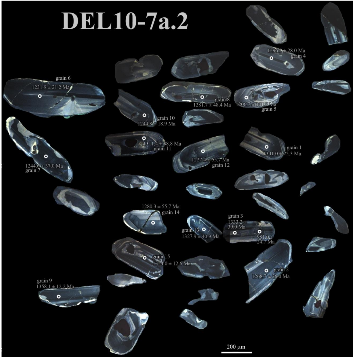
Figure 5.10: Cathodoluminescence images of zircon grains from tx-DEL10-7a.2. Rings represent 20 μm LA spot locations. Errors are 1σ.
