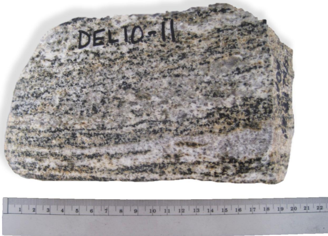
Figure 3.11: Slab sawn from hornblende gneiss sample DEL10-11 showing a distinct compositional banding defining foliation. Ruler units are cm.
