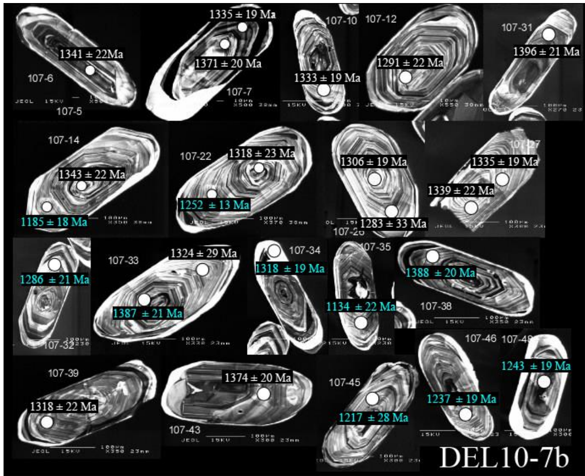
Figure 5.7: Cathodoluminescence images of zircon grains from sample hgn-DEL10-7b. Rings represent 20 \mu\text{m} SHRIMP II spot locations. Blue ages were not included in mean age calculation. Errors are 2\sigma .
