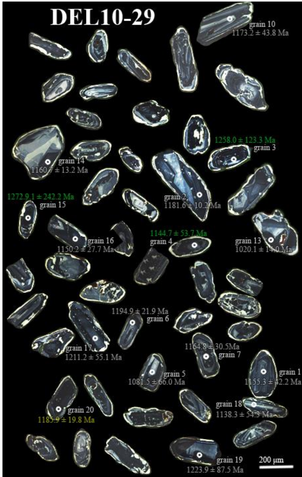
Figure 5.1: Cathodoluminescence images of zircon grains from agn-DEL10-29. Rings represent 20 μm LA spot locations. Green ages are analyses with anomalously high ^{204}\text{Pb} counts. Yellow ages are analyses with greater than 10 % ^{206}\text{Pb}/^{238}\text{U} error. These analyses were not included in the concordia or probability density plots. Errors are 1\sigma .
