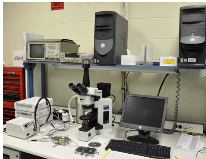
Figure 4.5: (a) Configuration of the hotstage microscopy system, (b) hotstage microscopy setup in the Brazing Research Laboratory of the University of Kentucky
