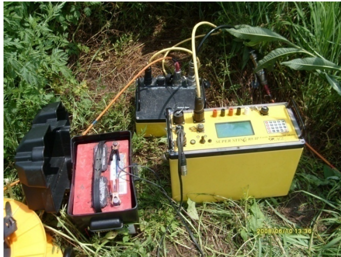
Figure 2.4. Eight-channel SuperSting R8/IP resistivity meter used for the survey.
