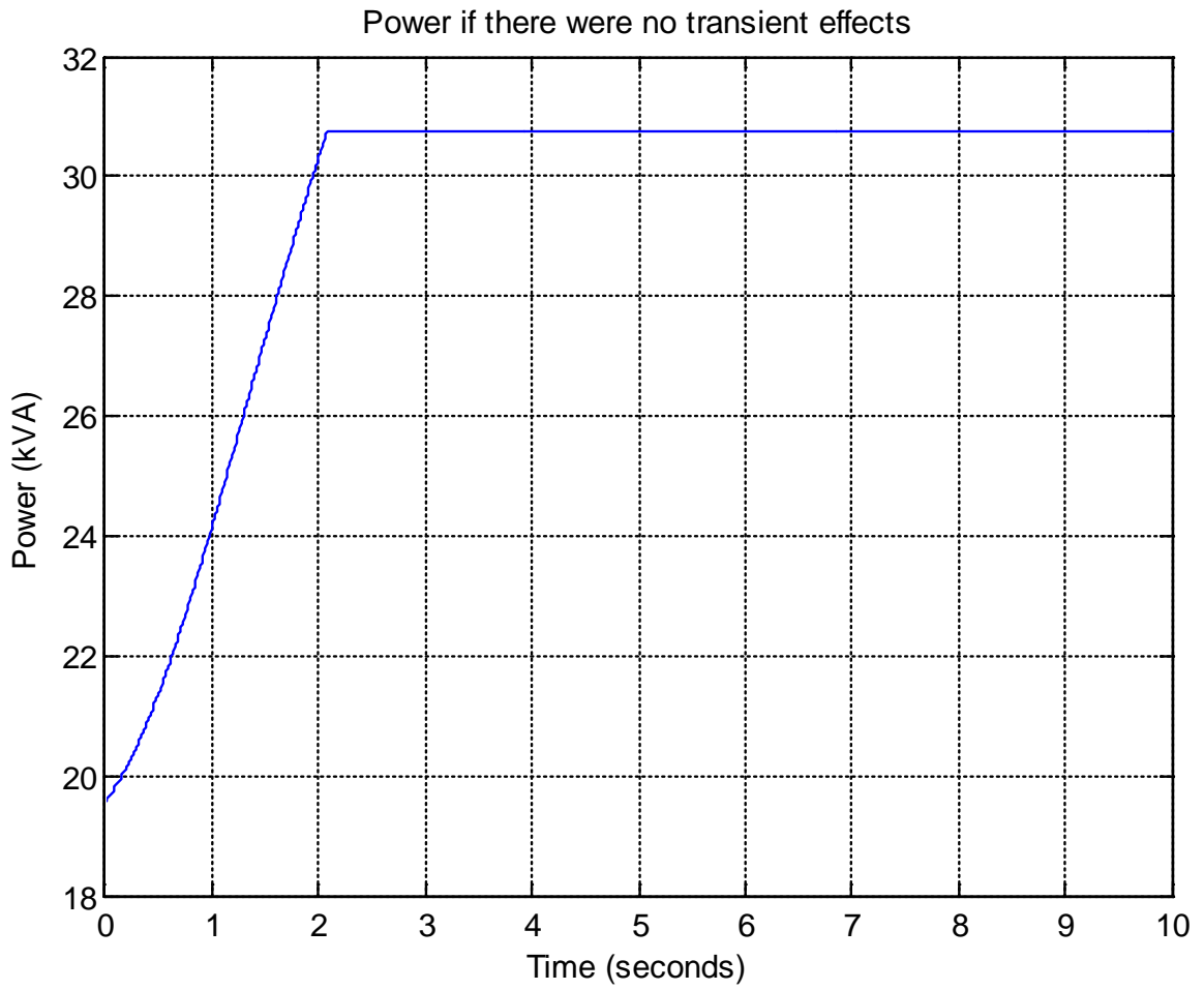
Figure 34: Total System Power if there was No Transient Effects in the Motor
