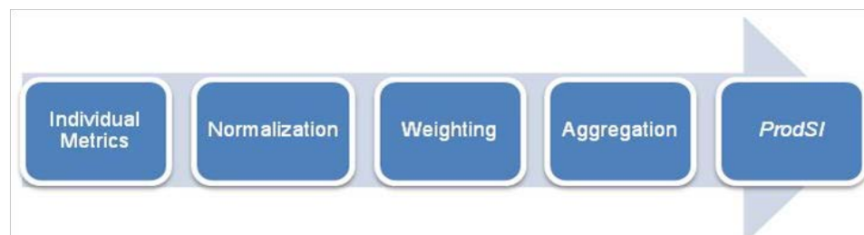
Figure 3-9 The five-step hierarchical ProdSI evaluation process
