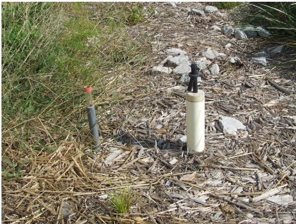
Figure 2.13: Picture of lysimeter and tensiometer in the rain garden at X1.
