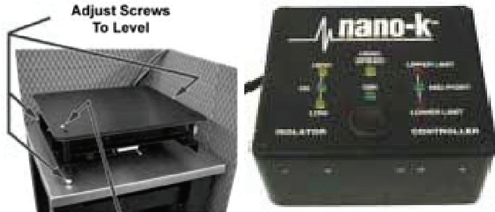
Figure 3-4 The Minus K Table (Left) minimizes external vibration excitations. The Nano-K auto-adjust system (Right) provides initial active damping and monitoring of harmonic oscillations, MTS [22].
