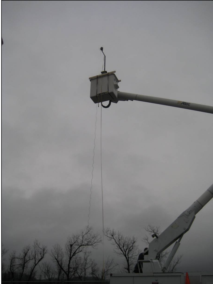
Figure 52 – KySat-1 Engineering Model Mounted to Bucket Truck
