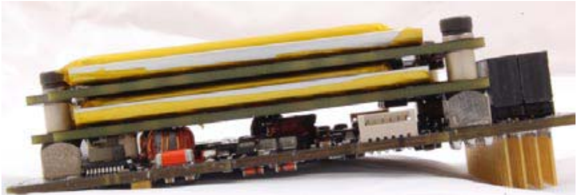
Figure 20 – Spacecraft Power System with Two Stacked Batteries
