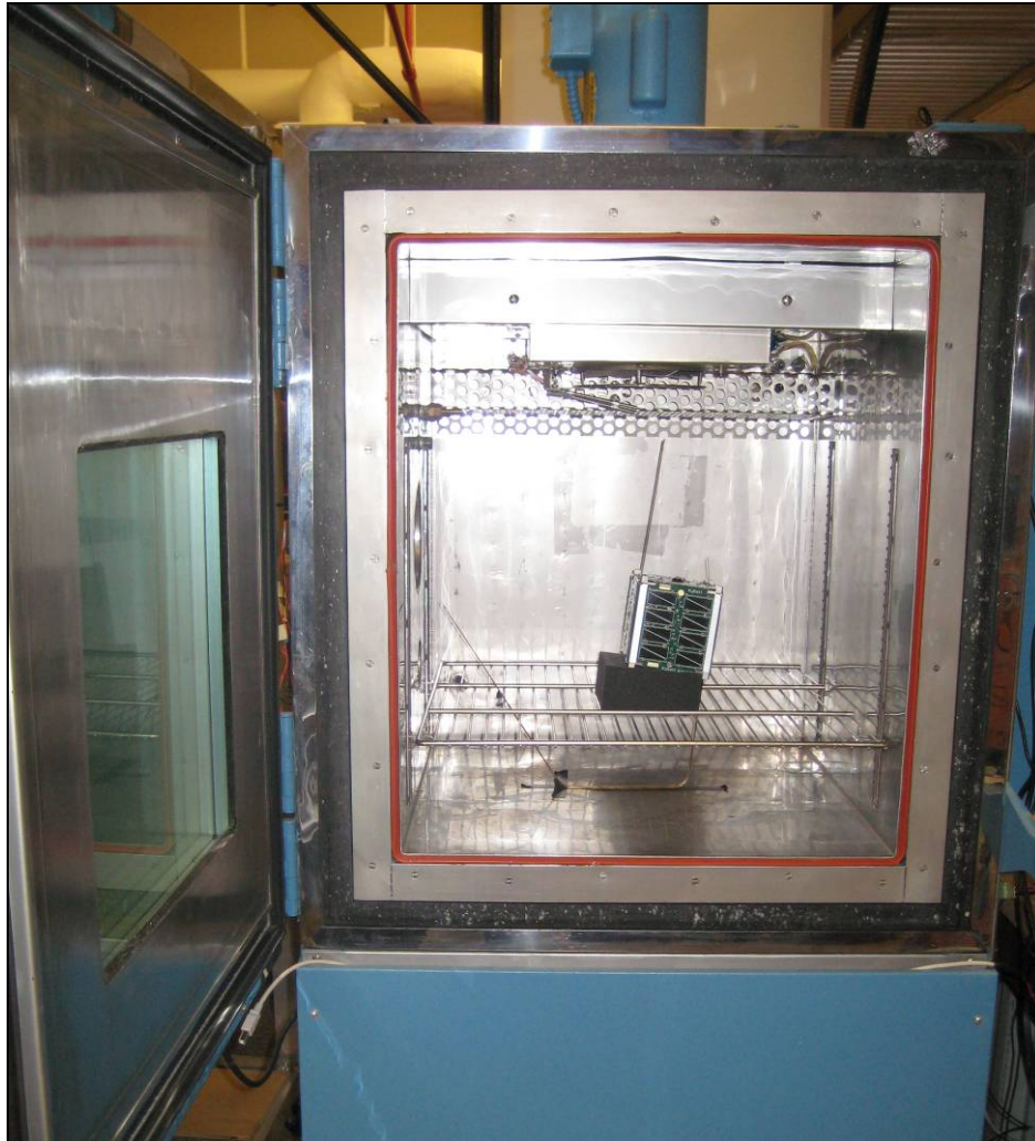
Figure 42 – KySat-1 Engineering Model inside the Thermal Chamber
