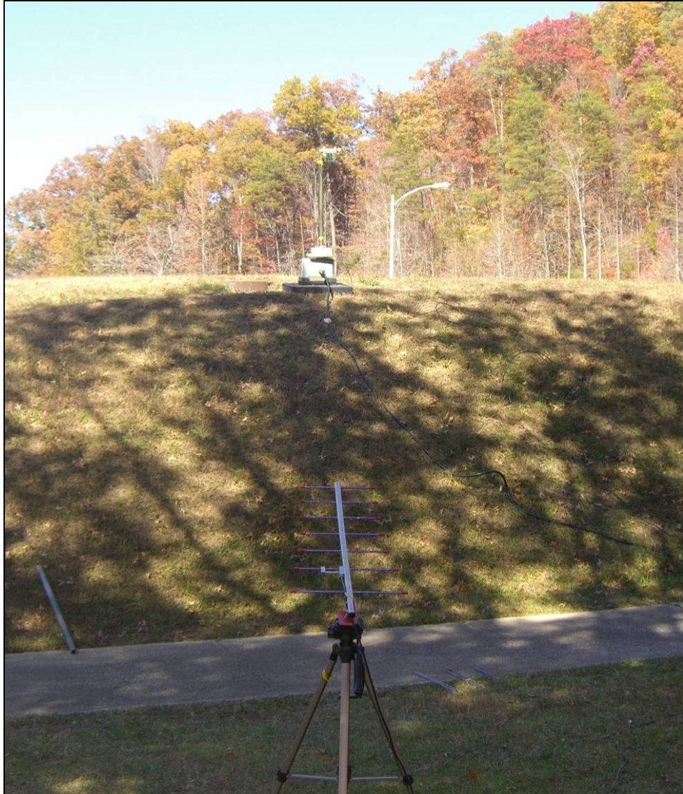
Figure 37 – Configuration used to Measure the Spacecraft Antenna Radiation Patterns
