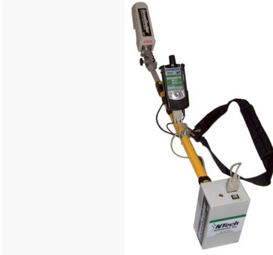
Figure 2.2: Handheld GreenSeeker proximal active reflectance sensor.
