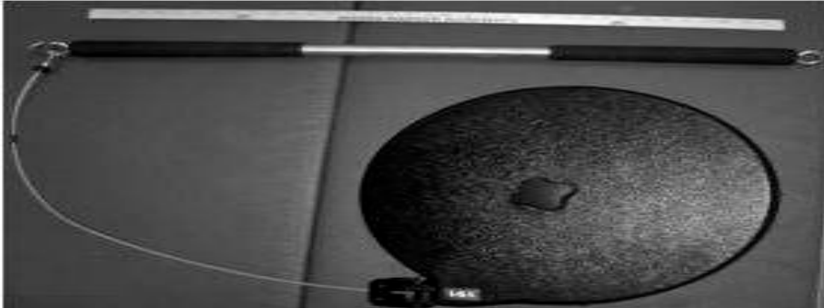
Figure 3.1: PrimusRS 3-dimensional cable motion system
