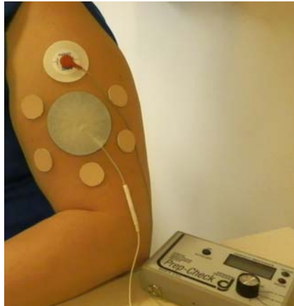
Figure 6.2 Treatment patches and electrodes on a subject's upper arm. The reference electrode was placed in the middle of all the treatment sites, which were protected during the study by blank occlusive patches. The top treatment site displays one of the Ag/AgCl measurement electrodes, which is moved from site to site to make impedance measurements. Both the reference and measurement electrodes are connected by lead wires to the impedance meter.
