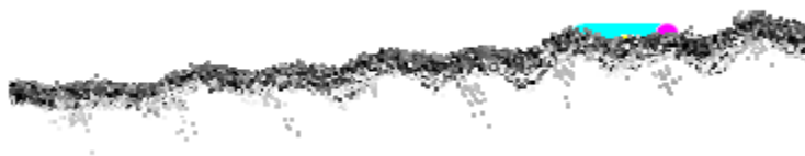
Figure 3.20 Measuring wavelength of the ripples of a smooth surface after PIL correction
