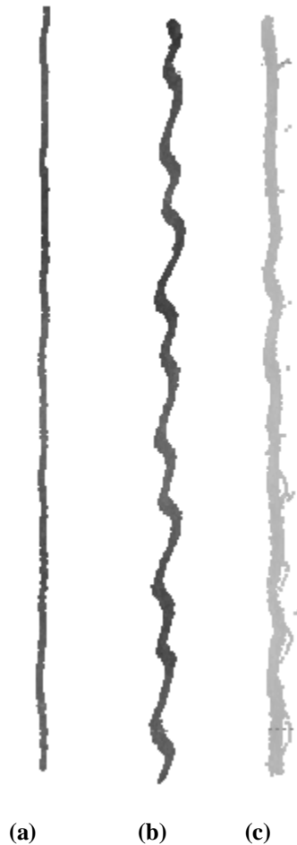
Figure 5.5 (a) cropped side view static 3D reconstruction of a smooth surface (b) cropped side view of the 3D reconstruction of the smooth surface which is subjected to non-uniform motion and (c) cropped side view of the 3D reconstruction of the smooth surface using PIL technique.
