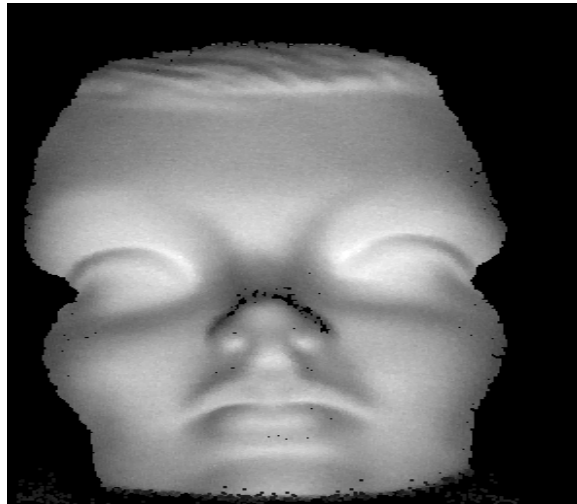
Figure 5.2 3D reconstruction of a face model
