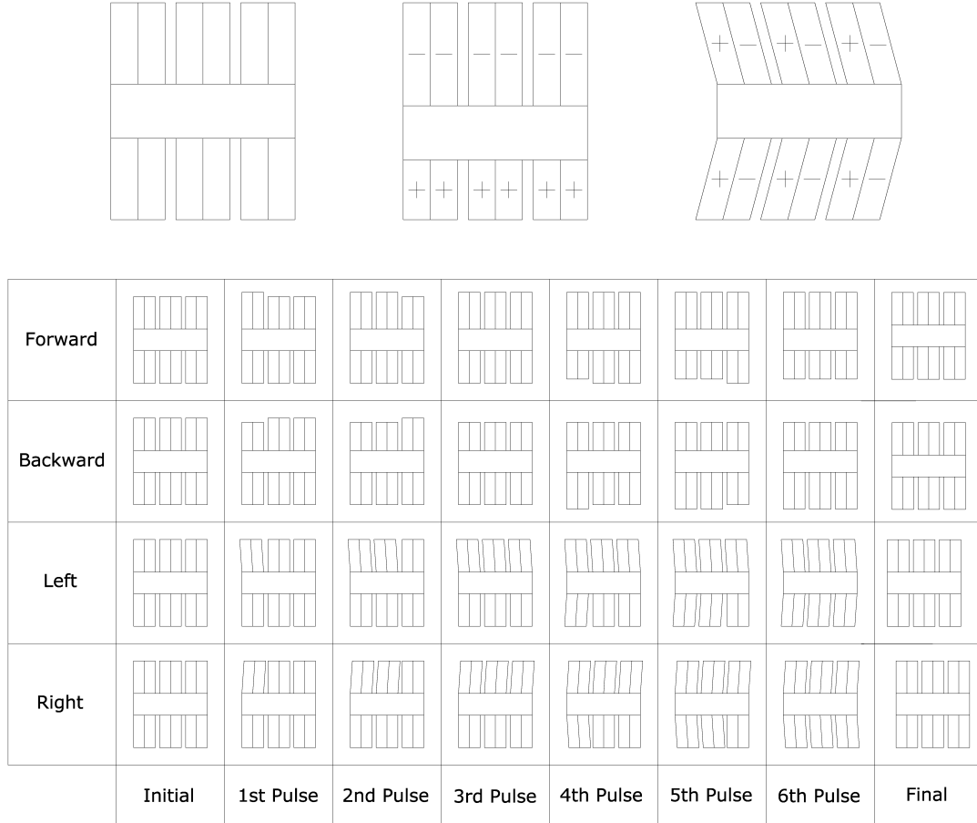
Figure 6.2: (top left) The walker assembly in the relaxed state with all electrodes held at ground potential. (top middle) The walker assembly with legs elongated and contracted for motion in the z-direction. (top right) The walker assembly with legs bent for motion in the x-direction. (Bottom) Diagram of how individual pulses are orchestrated to obtain net motion in all four directions.
