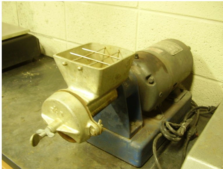
Figure 4.1 – Photograph of the disk mill used to grind raw materials.
