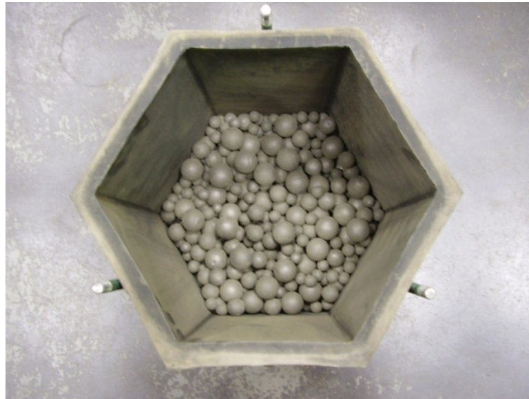
Figure 4.2 – Photograph looking down into the ball mill showing its cross-section and steel media used for grinding action.
