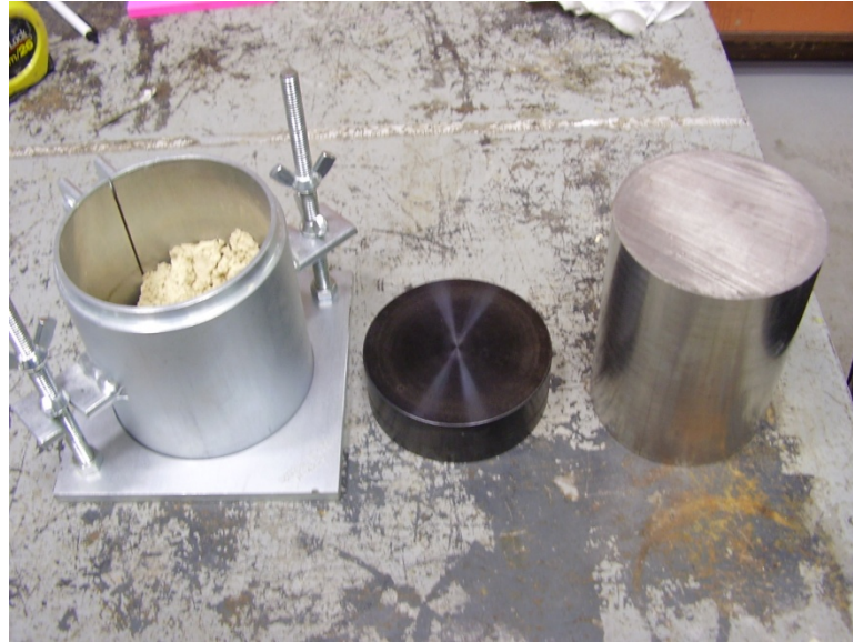
Figure 5.2 – Photograph of the items used to form the gypsum into molded bodies. Pictured from left: Proctor mold with moist FGD gypsum, short cylinder, and tall cylinder.
