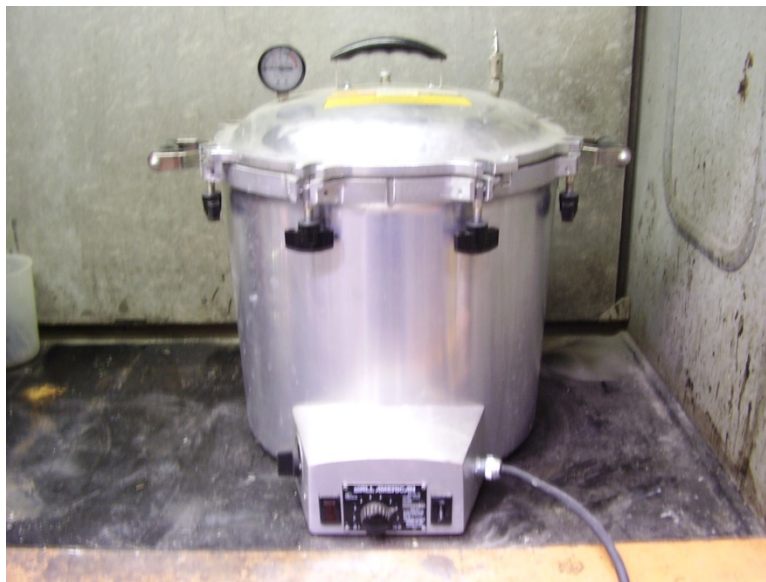
Figure 4.5 – Photograph of the All American Model 75X Pressure Steam Sterilizer used in the production of hemihydrate.
