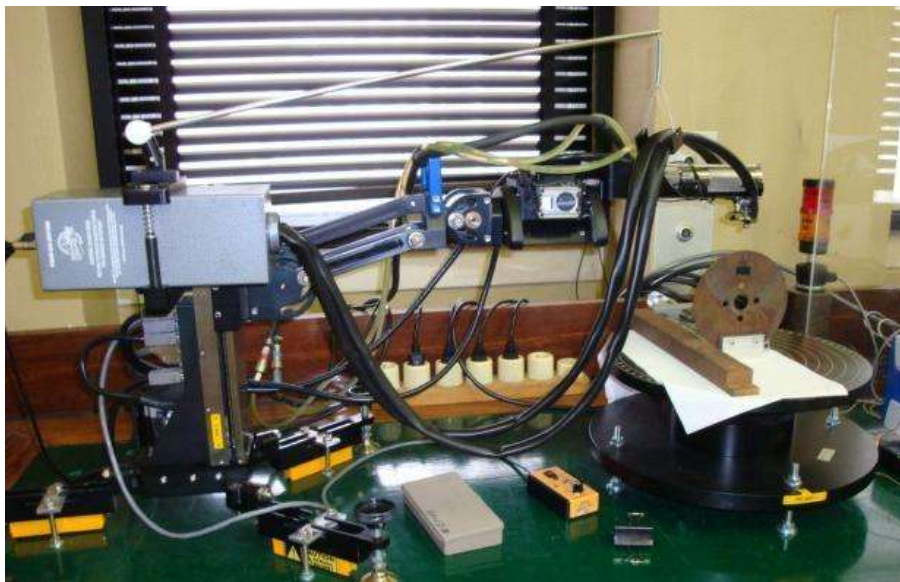
Figure 4.1: PROTO iXRD machine used in the residual stress measurement (X-ray Diffraction Center for Materials Research, University of Coimbra, Portugal)
