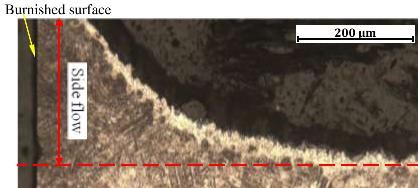
Figure 4.14: Material side flow after burnishing (cryogenic, 0.15 mm DoP, 100 m/min burnishing speed)
