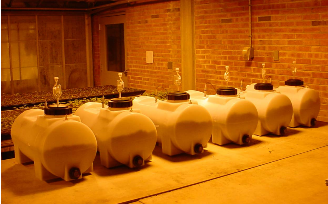
Figure 3.6 Picture of the tanks after being filled with the treatment material and the installation of the redox probe.
