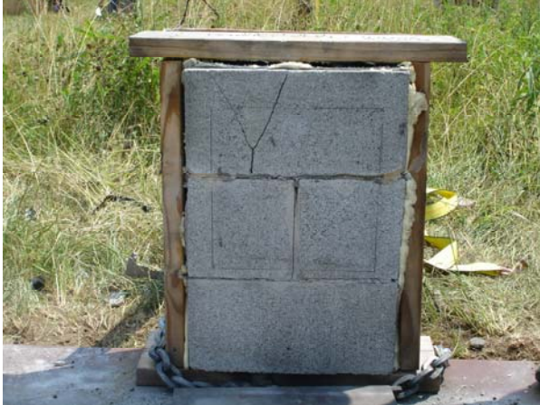
Figure C.12.a, b, c, d Blast 12 - 4lb. UFA & KFOAML1 (Clockwise from upper left) (a) Front of foam sample before blast; (b) Front of mock wall after blast; (c) Front of mock wall after blast.
