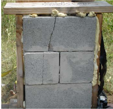
Figure 5.32 Result of Blast 16 – 8 lb. Ceno & 4 lb. Ceno (Cracked – Fail)
