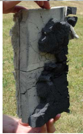
Figure C.6.a, b, c, d Blast 6 - 4lb.Ceno & 8lb.Ceno & KFOAML (Clockwise from upper left) (a) Front of foam sample before blast; (b) Front of mock wall immediately after blast. Some adhesive is visible; (c) Side view of foam sample remains after blast; (d) Front of mock wall after blast and after removing foam sample and steel plate.
