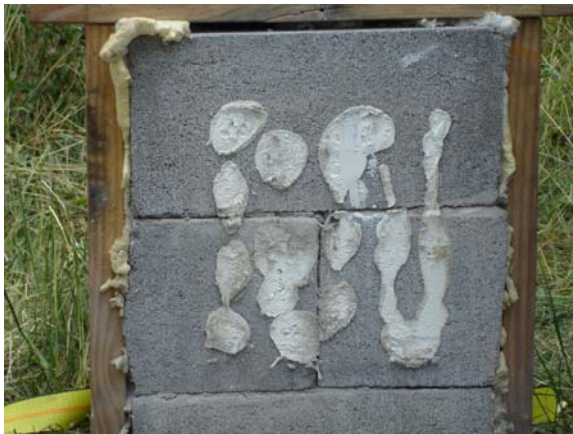
Figure C.8.a, b, c, d Blast 8 - 4lbCeno & 8lbUFA & KFOAML1 (Clockwise from upper left) (a) Front of foam sample before blast; (b) Front of foam sample after blast; (c) Front of mock wall after removing foam sample and steel plate. Some adhesive is visible; (d) Front of mock wall after blast.
