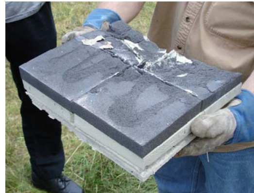
Figure C.5.a, b, c, d, e Blast 5 - 4lb.Ceno & 8lb.Ceno & KFOAML1 (Clockwise from upper left) (a) Front of foam sample before blast; (b) Front of foam sample immediately after blast; (c) Front of foam sample and steel plate after blast. Some adhesive is visible; (d) Thickness of entire hybrid composite sample. Area of blast damage was clearly off center.
