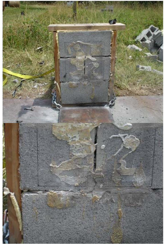
Figure C.16.a, b, c, d Blast 16 - 8lb.Ceno & 4lb.Ceno (Clockwise from upper left) (a) Front of foam sample before blast; (b) Front of mock wall after blast. Some adhesive is visible; (c) Front of mock wall up close after blast; (d) Front of mock wall after tilting parallel with ground after blast.
