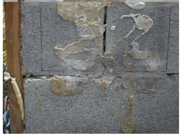
Figure C.16.a, b, c, d Blast 16 - 8lb.Ceno & 4lb.Ceno (Clockwise from upper left) (a) Front of foam sample before blast; (b) Front of mock wall after blast. Some adhesive is visible; (c) Front of mock wall up close after blast; (d) Front of mock wall after tilting parallel with ground after blast.
