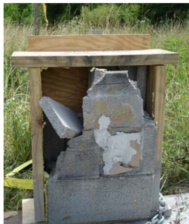
Figure 5.18 Result of Blast 2 – 2 Layers of Drywall (Broken – Fail)
