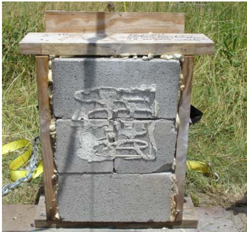
Figure C.6.a, b, c, d Blast 6 - 4lb.Ceno & 8lb.Ceno & KFOAML (Clockwise from upper left) (a) Front of foam sample before blast; (b) Front of mock wall immediately after blast. Some adhesive is visible; (c) Side view of foam sample remains after blast; (d) Front of mock wall after blast and after removing foam sample and steel plate.
