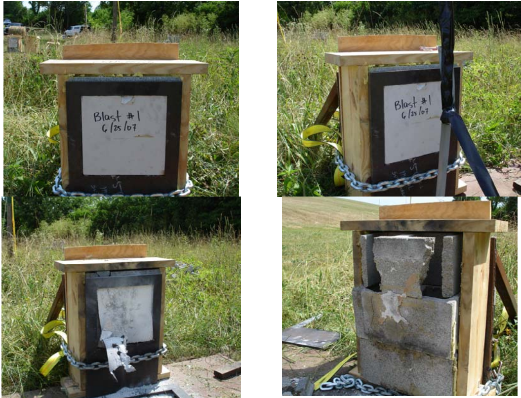
Figure C.1.a, b , c, d Blast 1 – Drywall Only (Clockwise from upper left) (a) Front of dry wall only sample before blast test; (b) C4 charge positioned in front of the foam sample held in position by tape; (c) Front of foam sample immediately after blast; (d) Mock wall condition after foam sample and steel plate were removed.
