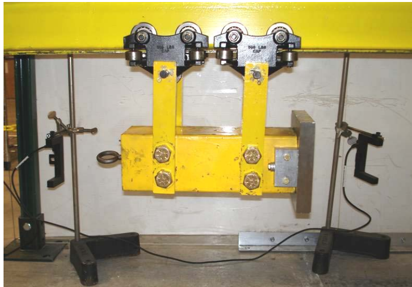
Figure 1.2 Final Impact Sled Used During Middle Strain Rate Tests. (Light gates that obtain the sled speed are shown.)
