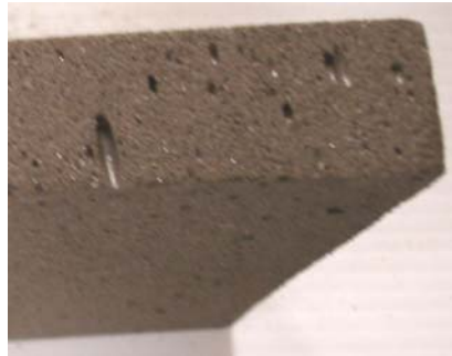
Figure 3.3 Elongated pores formed in 8 lb. polyurethane foam with cenospheres
