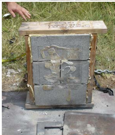
Figure C.16.a, b, c, d Blast 16 - 8lb.Ceno & 4lb.Ceno (Clockwise from upper left) (a) Front of foam sample before blast; (b) Front of mock wall after blast. Some adhesive is visible; (c) Front of mock wall up close after blast; (d) Front of mock wall after tilting parallel with ground after blast.
