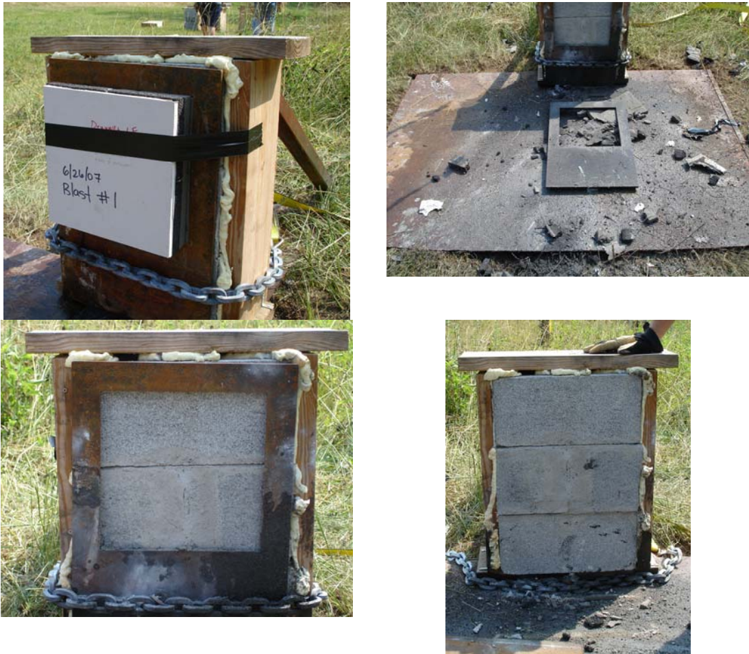
Figure C.9.a, b, c, d Blast 9 - 4lb.UFA & 8lb.UFA & KFOAMLF (Clockwise from upper left) (a) Front of foam sample before blast; (b) Condition of experimental setup area after 9 blasts; (c) Front of mock wall after foam sample and steel plate are removed after blast; (d) Front of mock wall after blast.
