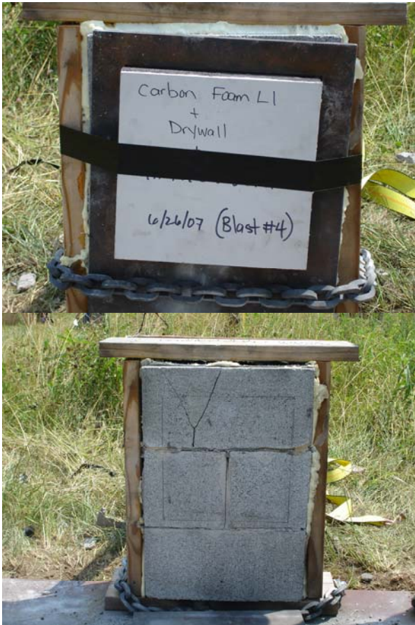
Figure C.12.a, b, c, d Blast 12 - 4lb. UFA & KFOAML1 (Clockwise from upper left) (a) Front of foam sample before blast; (b) Front of mock wall after blast; (c) Front of mock wall after blast.
