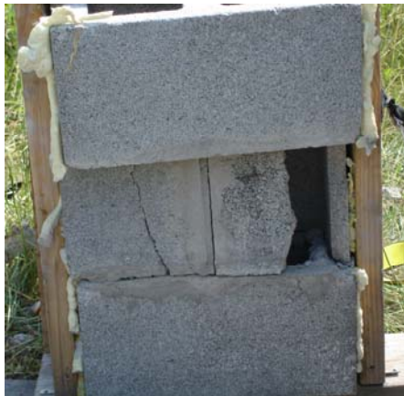
Figure 5.17 Result of Blast 11 – Polystyrene Foam & 8 lb. Ceno & KFOAML1 (Broken – Fail)
