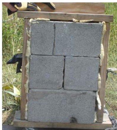
Figure 5.31 Result of Blast 15 – 8 lb. Ceno & KFOAML1 (Cracked – Fail)
