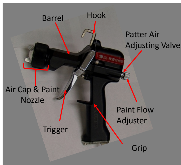
Figure 3.13: A picture of the HVLP air-assisted atomizer.
