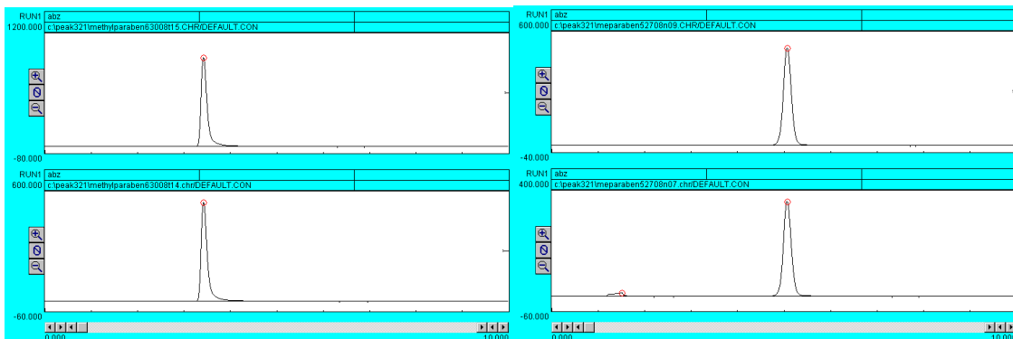
Figure 3.11a, Reverse phase HPLC chromatograms of methylparaben: the top chromatogram is the standard solution with drug concentration of 107ug/mL; the bottom curve represents 40-fold dilution of the saturated drug in 2.5mg/mL SDS solution.
