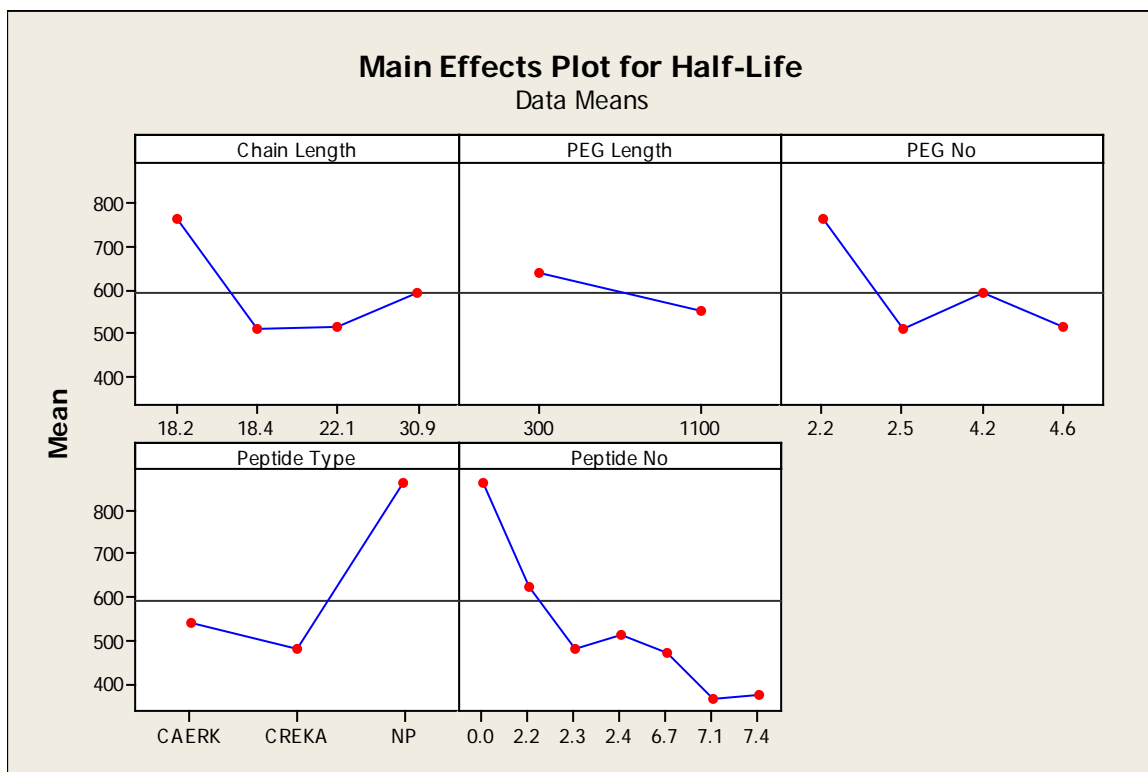
Figure 6-12 Main effects plots for the kinetic half-life of second fibrinogen adsorption step.
