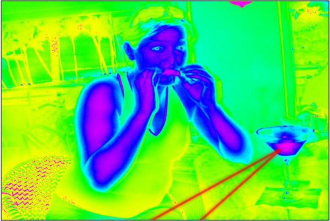
Figure 3.1: Remote alcohol sensing: a hypothetical situation where NIR laser beam is used to monitor speech from the glass on the table. MFC-NIR hyperspectral imaging is used for laser positioning and to determine the subject's BAC.
