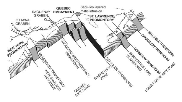
**Figure 4.2.** Schematic block diagram illustrating the 3-D structure of the eastern Laurentian rifted continental margin of northeastern North America (present coordinates) in the context of a low-angle detachment rift system (see Chapter 2). SILMI = Sept-Iles layered mafic intrusion.
