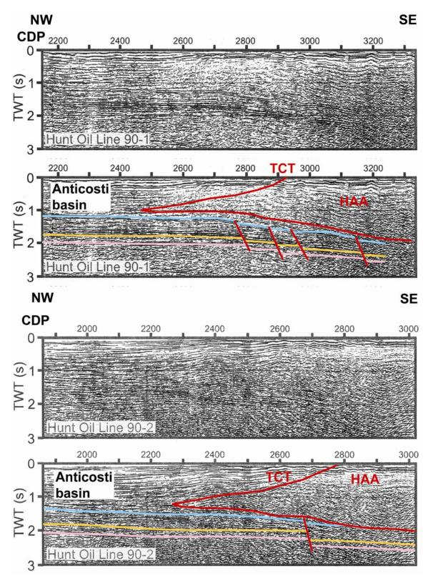
**Figure 3.19.** Uninterpreted and interpreted seismic data, Hunt Oil Co., lines 90-1 and 90-2. See Figure 3.7 for location. Color for interpreted stratigraphic and structural contacts same as Figure 3.13. Lines modified after Stockmal et al., (1998).
