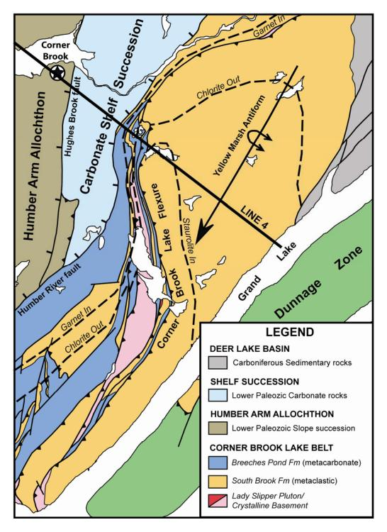
**Figure 3.23.** Generalized geologic map of the Corner Brook Lake terrane and surrounding geology. Map illustrates the distribution of rock types in the terrane, along with significant structures and metamorphic isograds (dashed lines). Note the contrasting geology around the Corner Brook Lake flexure. Modified after Cawood and van Gool (1998).
