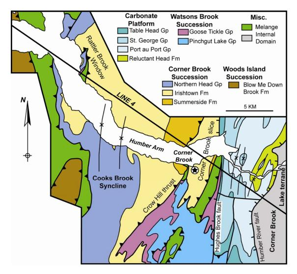
**Figure 3.18.** General geologic map of the Humber Arm allochthon and underlying platform rocks in the area of Corner Brook and Humber Arm. Figure displays significant structural slices within the allochthon in region, significant map scale structure, and part of cross-section Line 4. Geologic map based on previously published maps by Knight (1996), Waldron et al (2003), and geologic mapping by the author.
