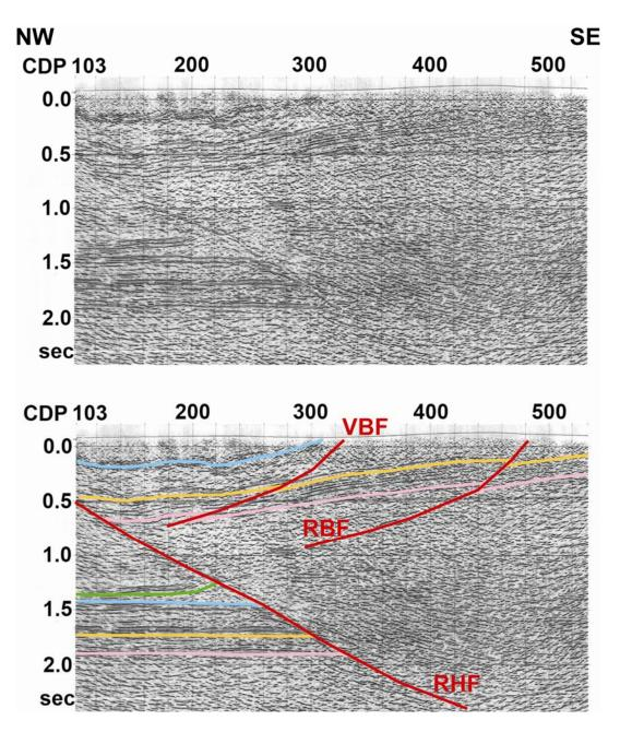
**Figure 3.14.** Uninterpreted and interpreted seismic data, Hunt Oil Co. line 93-7. Significance of individual line colors same as in Figure 3.13. The Mainland Sandstone occupies the region between the light blue and dark green seismic reflectors. Note that in this seismic profile the thickness of reflectors correlated to the Mainland Sandstone is greater in the hanging wall of the Round Head fault than in the footwall. RBF = Red Brook fault; RHF = Round Head fault; VBF = Victors Brook fault.
