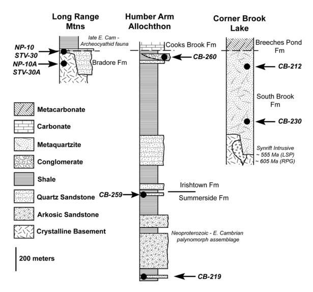
**Figure 4.3.** Stratigraphic sections across the Humber zone illustrating the late Neoproterozoic-Early Cambrian synrift stratigraphy in the parautochthon (Long Range Mtns), the Humber Arm allochthon, and in the eastern internal domain (Corner Brook Lake). Sample locations identified by sample numbers and illustrated (black circles) with respect to location in the vertical stratigraphic section.
