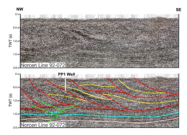
**Figure 3.28.** Uninterpreted and interpreted seismic data, Norcen line 92-072. See Figures 3.7 and 3.25 for location. Color for red, pink, and light blue lines same as Figure 3.13. Yellow lines indicate stratigraphic contact between the Cow Head Group and the Lower Head Formation in the Humber Arm allochthon. Green lines illustrate a late "pop-up" structure that deforms the shelf succession and overlying Humber Arm allochthon. PP1 = Parsons Pond Well #1.
