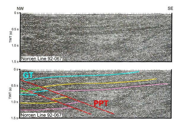
**Figure 3.26.** Uninterpreted and interpreted seismic data, Norcen line 92-067. See Figures 3.7 and 3.25 for location. Color for interpreted stratigraphic and structural contacts same as Figure 3.13. GT = thick section of Goose Tickle Group; PPT = Parson's Pond fault.
