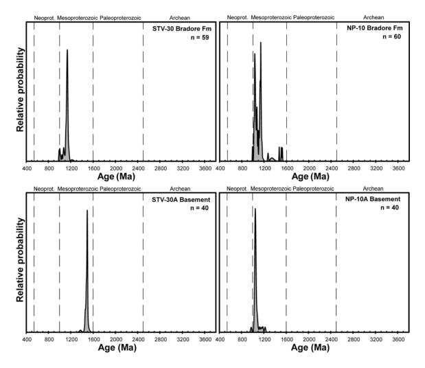
**Figure 4.4.** Cumulative probability density diagrams for U-Pb isotopic ages in zircon from the basement-cover samples. Only those analyses within  $\pm 10\%$  discordance are plotted.
