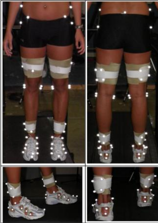
Figure 3.1 Marker set used during a static calibration. Only bilateral markers on the lateral aspects of the 5 th metacarpal head, base, navicular and both the lateral and medial aspects of the calcaneus were used to model foot movement. Windows are cut out of the shoes allowing markers to be adhered directly to the foot. Rigid clusters were secured to the distal posterior-lateral aspects of each segment to model thigh and shank movement.
