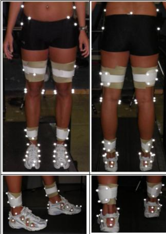
Figure 4.1 Markerset used during a static calibration. Only bilateral markers on the lateral aspects of the 5 th metacarpal head, base, navicular and both the lateral and medial aspects of the calcaneus were used to model foot movement. Windows are cut out of the shoes allowing markers to be adhered directly to the foot at locations consistent with Pohl et al.(Pohl, et al. 2007). Rigid clusters were secured to the distal posterior-lateral aspects of each segment to model thigh and shank movement.
