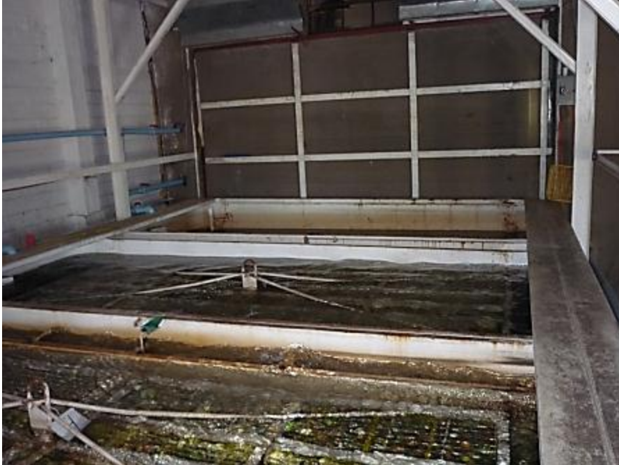
Figure 6-6 HWT unit, "batch (Jacuzzi)" type Unlike in the “continuous” type, a basket does not move during treatment but stays in a separate tank. When a treatment is finished, the basket will be hoisted and moved beyond the screen wall (behind the last tank) for packing in Sinaloa, Mexico (Photo by author)
