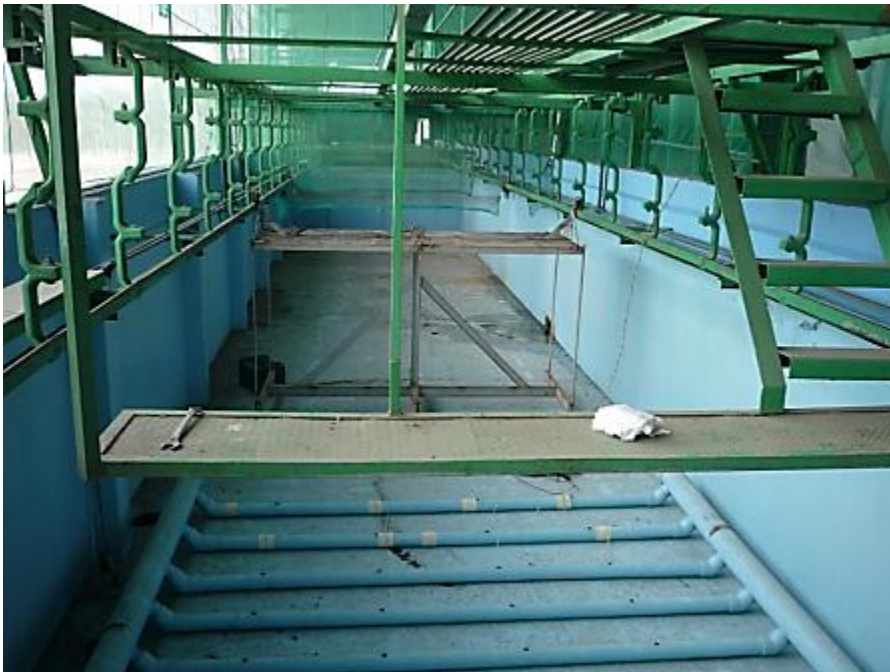
Figure 6-5 Continuous HWT unit (the last one in Mexico) in Escuinapa, Mexico A basket, hanging from above (like a gondola lift), moves from this side towards the opposite end in the trench, which will be filled with hot water when in use (Photo by author)
