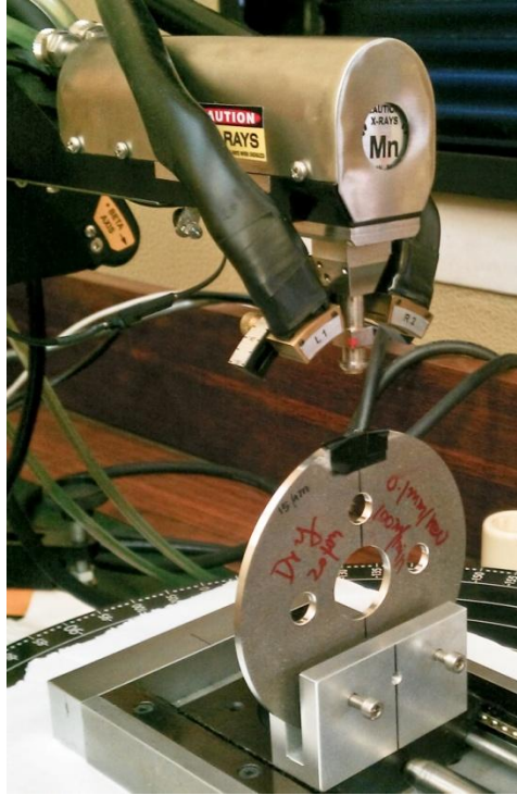
Figure 3.3: Experiment setup at the University of Coimbra (Portugal) for residual stress measurements on machined AZ31B Mg discs using iXRD from PROTO®
