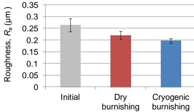
Figure 4.16: Surface roughness ( R_a ) before and after burnishing under dry and cryogenic conditions.
