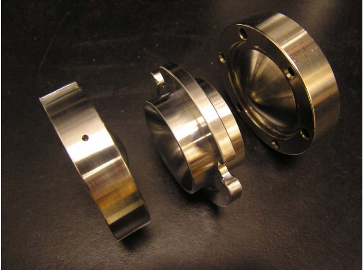
Figure 2-7: Ion trap mass spectrometer
