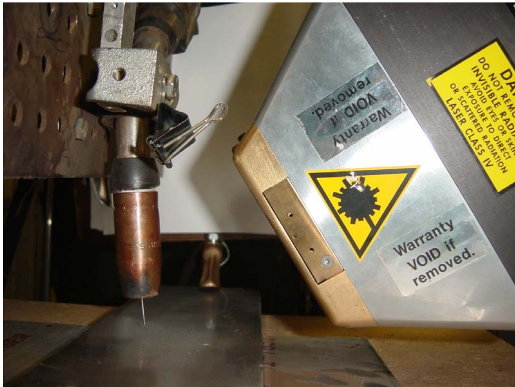
Fig. 3-3 Installation of GMAW and Laser (the shielding board is not shown in the picture)
